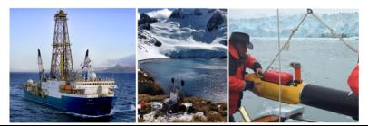
UTIG applies an array of platforms and methods to address problems in marine geosciences, seismology and tectonics including IODP drilling (left), GPS reference stations (center), multibeam swath mapping, multi-channel seismic imaging, ocean bottom seismometers (cover image) and develops new avenues for acquisition with emerging tools such as Autonomous Underwater Vehicles (right).
