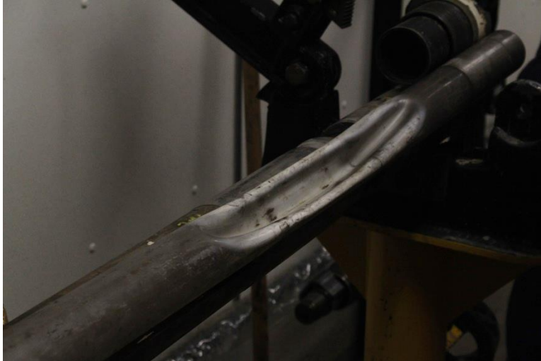
Figure 4: Collapsed liner after Flow Test 3.
