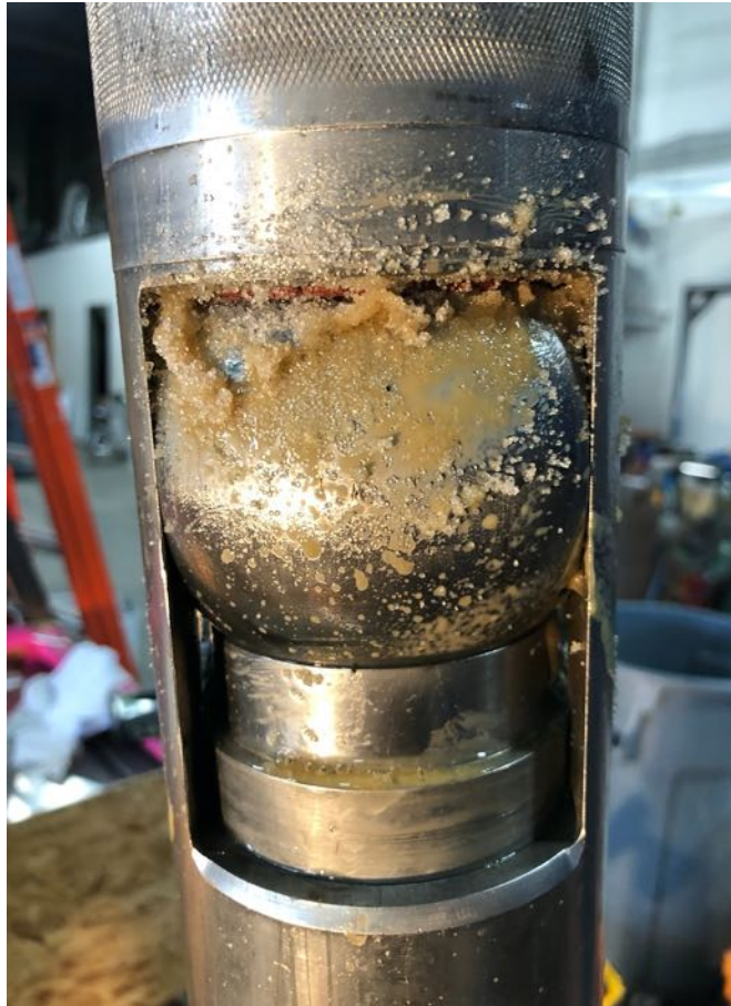
Figure 19. Ball valve covered with #100 mesh sand
