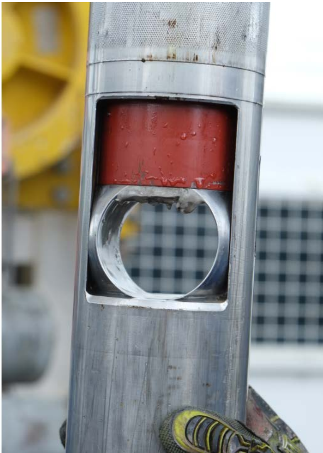
Figure 5-7. Illustration of an apparently closed ball valve upon recovery from the hole. Although it is apparently sealed, no pressure was held. It is interpreted that either it was a leaky seal or that the ball valve closed after the pressure was boosted. Note the mud and silt between the ball and the seal carrier (red).
