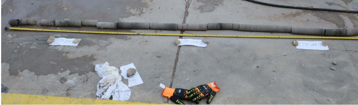
Figure 2: Core CTTF-2FB: 2.7 m of core were recovered composed of light grey resistant carbonate and more fissile charcoal colored shale.
