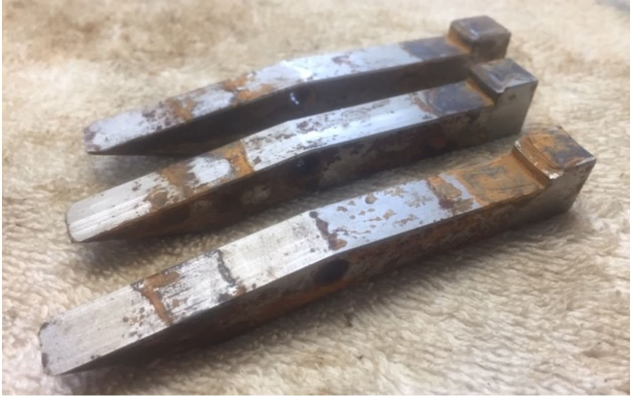
Figure 4-5. Upper latch dogs with brinelled heels
