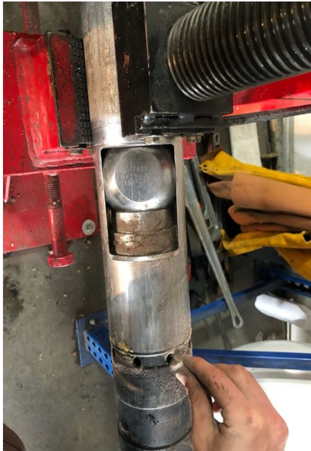
Figure 20. Ball valve assembly with applied Aluminum Oxide
