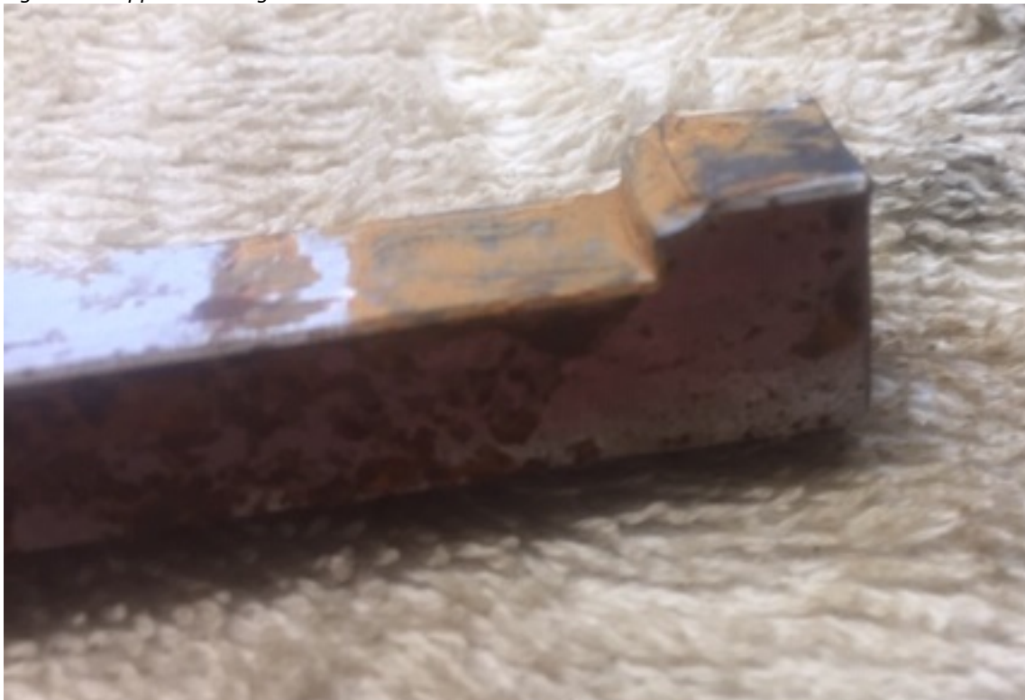
Figure 4-6. Close up of upper latch dog brinelled heel.
