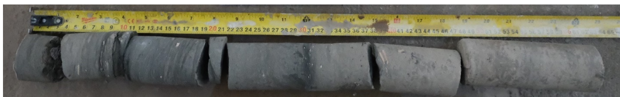
Figure 5-3. Core CTTF-04CS is a high-quality core from the cutting-shoe tool. The pressure was not maintained in the sample, but that core had high recovery (80%) and had good quality.
