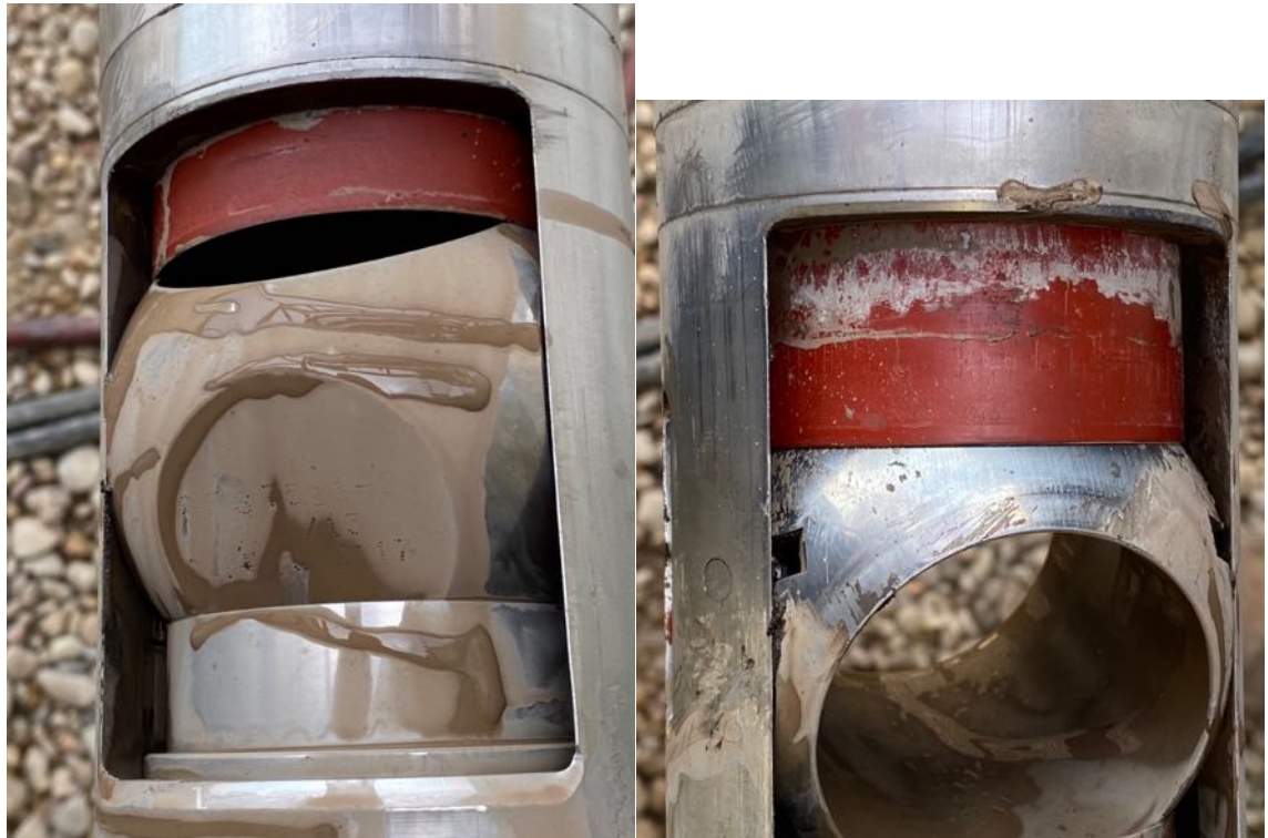
Figure 8. Seal carrier (red part), ball valve and ball follower after coring run 4CS. On recovery to the coring van (L) and after hammering to move the ball and sleeve (R). Note the material above the 'tide' mark on the seal carrier and the streaks close to the edge of the ball housing.
