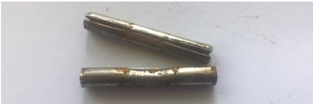
Figure 4-4. Deformed pivot and retaining pins.
