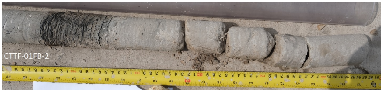
Figure 0-1 CTF-01FB from core run 1 (face-bit).
