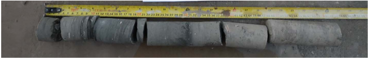
Figure 2: Core CTTF-04CS: 0.62 m of core were recovered composed of light grey resistant carbonate and charcoal colored shale.
