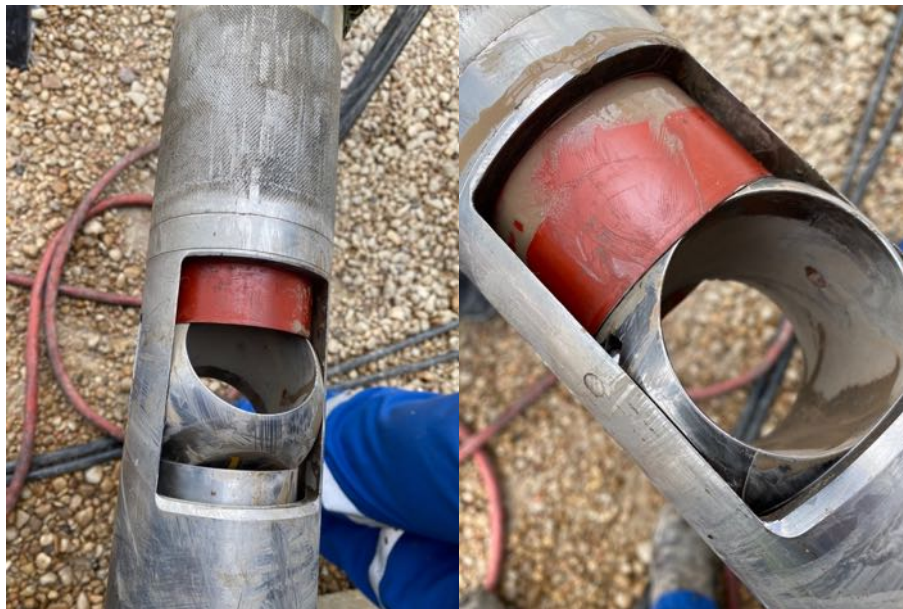
Figure 13. Ball valve, seal carrier (red part) and ball follower after Core Run 6CS. Note that the ball was moveable by hand suggesting that the seal carrier or spring was jammed above it. Note the coarse-grained looking material after the seal carrier has been moved down.
