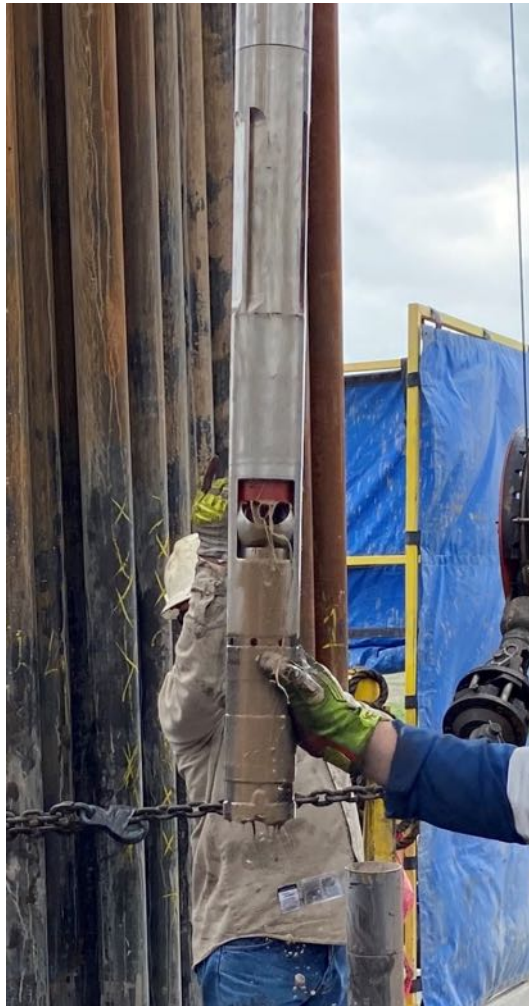
Figure 6. Seal carrier (red part), ball valve and ball follower (below the ball valve) after coring run 3CS.
