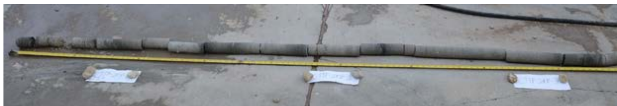
Figure 5-1. Core CTTF-02FB contained 8.9 ft of limestone and shale after recovery.
