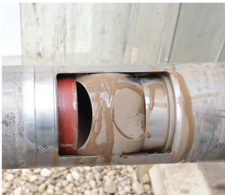
Figure 5-6. Illustration of a partially closed ball valve after recovery from the hole. The red object is the seal carrier. When the PCTB is actuated, a spring to the left of the seal carrier drives the seal carrier downward, which in turn drives ball downward (to the right). When the ball is forced downwards, it rotates around a pin into the closed orientation, sealing the bottom of the autoclave.
