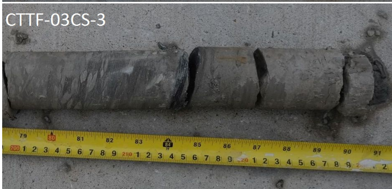
Figure 0-3 CTTF-03CS from core run 3 (cutting-shoe).
