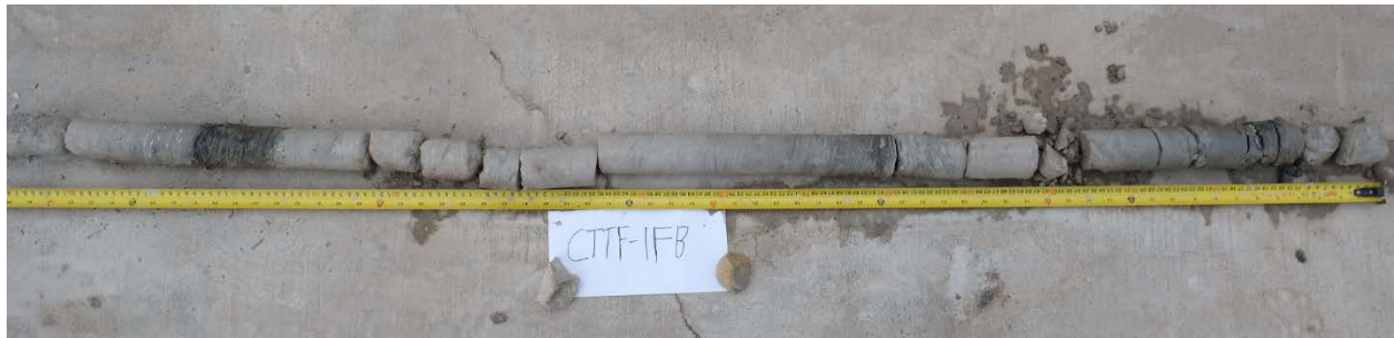
Figure 1: Core CTTF-1FB: 1.78 m of core were recovered composed of light grey resistant carbonate and more fissile charcoal colored shale.
