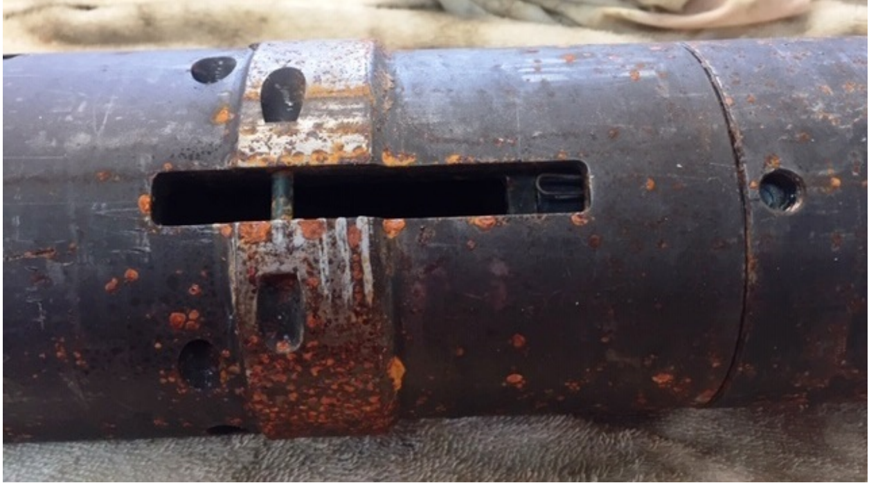
Figure 4-2. Missing locking dog.
