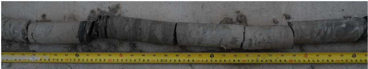
Figure 1: Core CTTF-03CS-2: 2.30 m of core were recovered composed of light grey resistant carbonate and more fissile charcoal colored shale.
