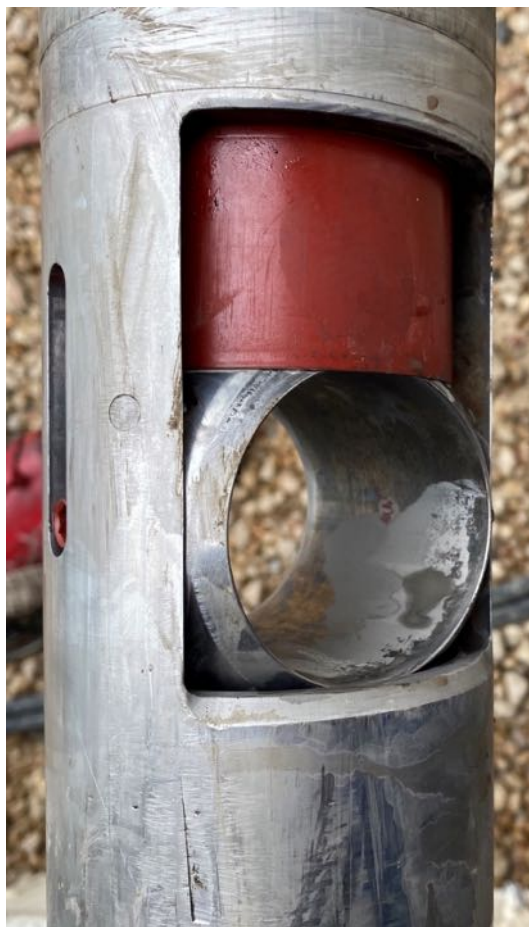
Figure 11. Seal carrier (red part), ball valve and ball follower after coring run 5CS. The ball is in the closed position and was most likely jostled into this position during handling at or from the rig floor.
