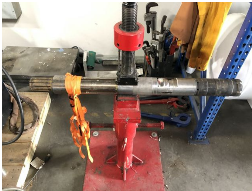
Figure 17. Isolated ball valve assembly for dry firing.
