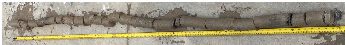
Figure 4. Core recovered during coring run 3CS.
