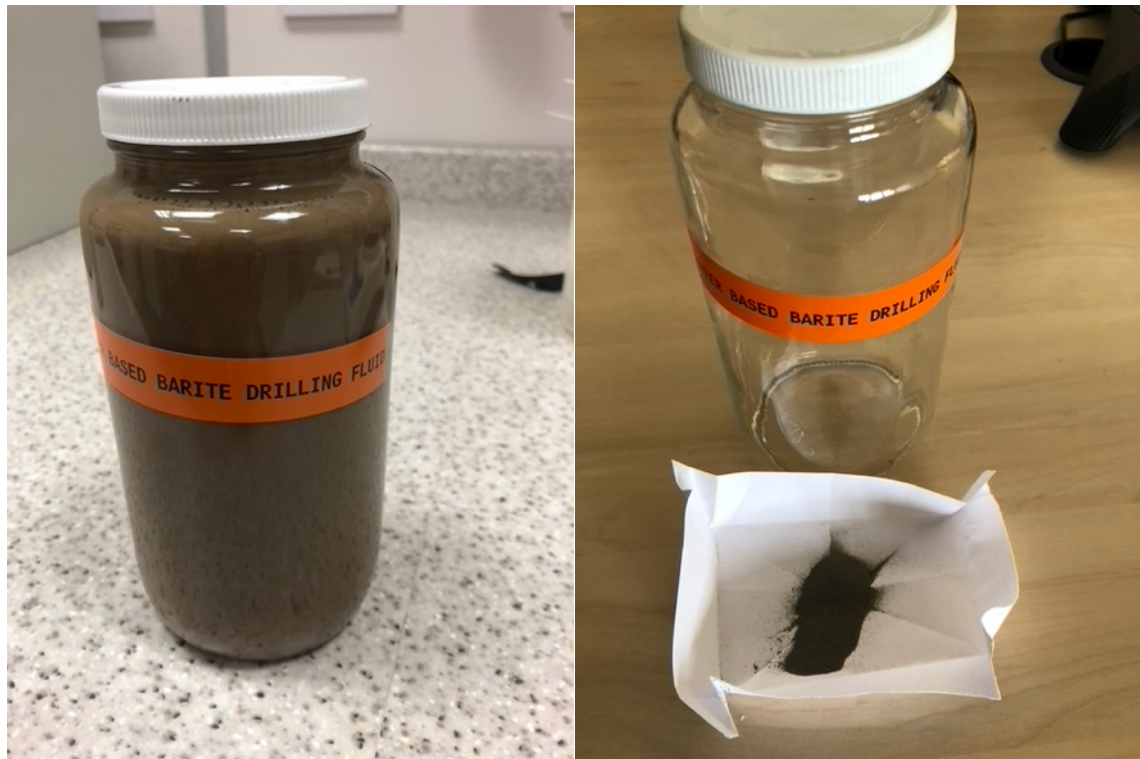
Figure 16. Mud sample from CTTF (L) and the coarse-grained material sieved from the mud (R).
