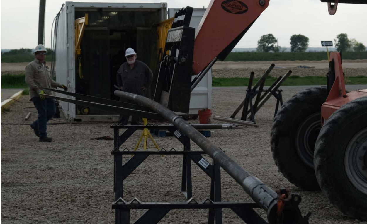
Figure 2: The Probe Deployment Tool (PDT) after it is made up prior to running in the hole.
