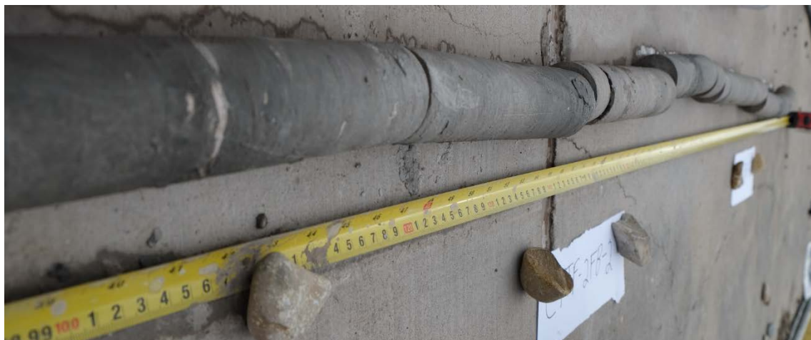
Figure 5-2. A closer view of Core CTTF-02FB. The core is consistent in diameter between limestone (light-colored intervals) and shale (dark-colored intervals). Most biscuits are tens of cm in length and very minor spiral grooves are visible.
