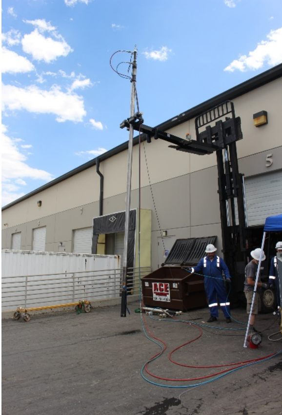
Figure 1.4: PCTB actuated hydraulically from top to simulate pull on wireline
