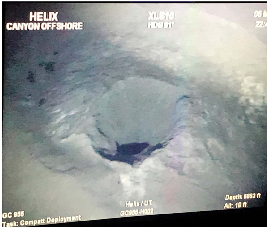
Figure 1.3.1. The H001 hole, drilled in 2009 during the Chevron JIP was found at the start of the UT-GOM2-01 Expedition. The hole is in remarkably good condition given that it was drilled 8 years before this photograph was taken.
