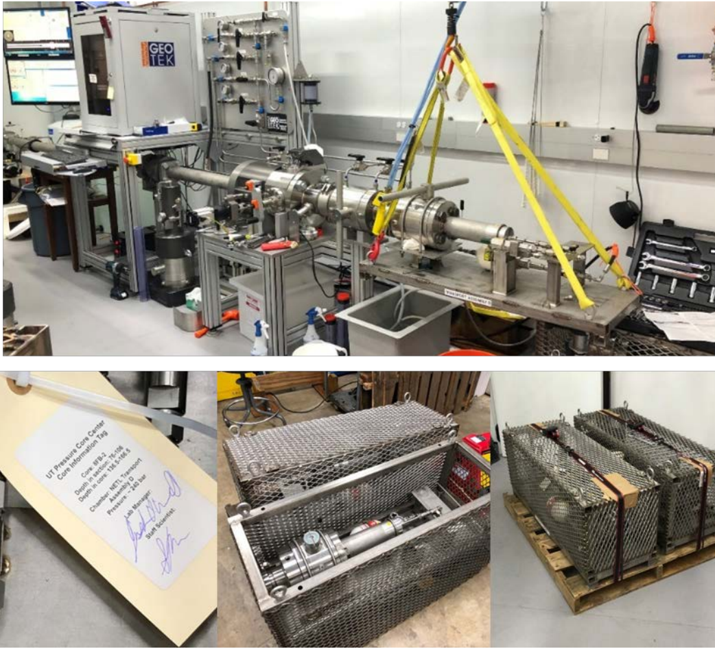
Figure 1-10: Images from the Pressure Core transfer from UT to NETL. Top, NETL storage and transfer chamber attached to UT Mini-PCATS. Lower left, chamber tagged w/ core info, certified by PCC lab manager and staff scientist. Lower center and lower right, NETL storage chambers ready for transfer to reefer van.
