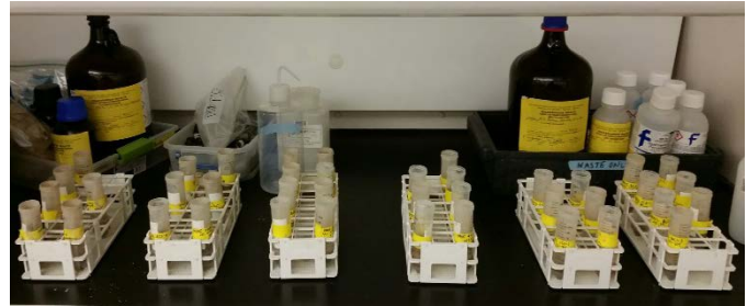
Figure 1-14: Sediment samples receiving hydrogen peroxide treatments in the chemical hood to remove organic carbon prior to measurement
