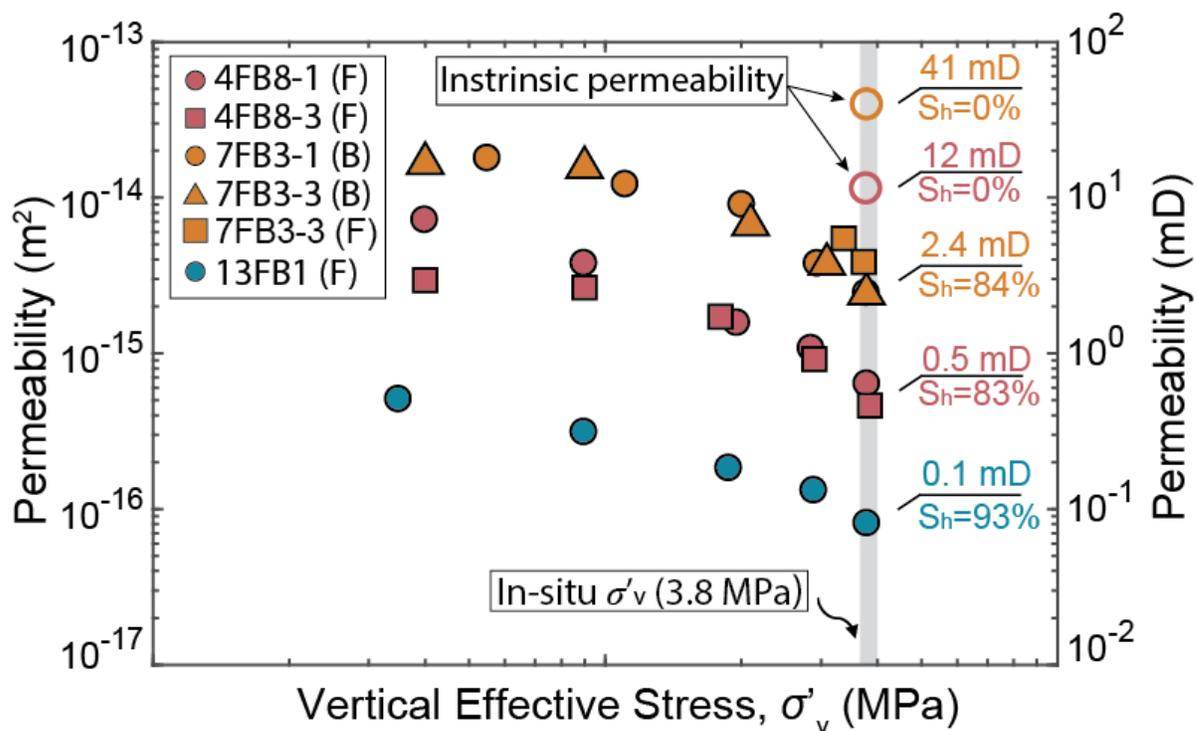
Figure 1-4: Permeability of UT-GOM2-1 Sandy silt sediment from three pressure core sections as a function of vertical effective stress before (effective permeability). The intrinsic permeability is measured by reconstitution approach. B-brine (3.5% salinity), F-freshwater.
