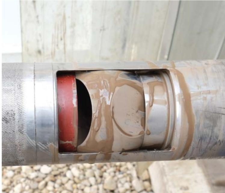
*Figure 1-9: Illustration of a partially closed ball valve after recovery from the hole. The red object is the seal carrier. A spring to the left of the seal carrier drives the ball downward (to the right). When the ball is forced downwards, it rotates around a pin and seals in place.*
