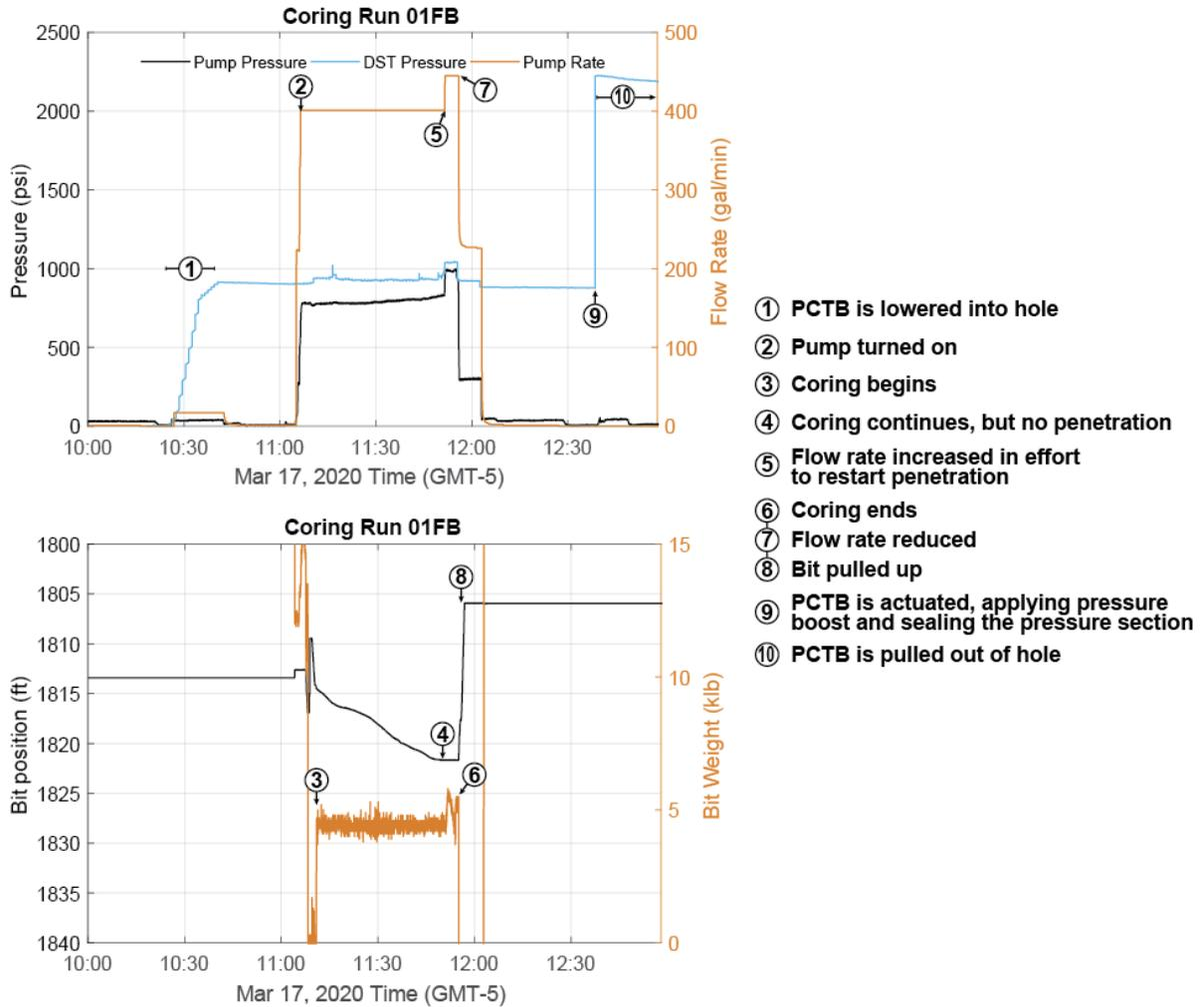
Figure 1-8: Autoclave (DST) pressure plotted alongside several rig parameters for the single core test in which pressure boost was successfully recorded and maintained (CTTF-01FB).
