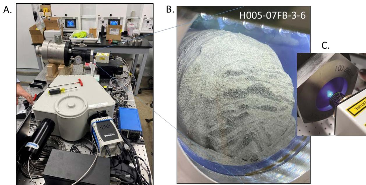
*Figure 1-5: micro-Raman spectrometer set up in the UT Pressure Core Center A. micro-Raman Pressure chamber connected to a Horiba Raman system (Lin). B. Hydrate-bearing sediment as seen through sapphire window of micro-Raman Pressure chamber. C. Photo of the Horiba Raman system lens next to the sapphire window during imaging using a blue laser (wavelength 473 nm).*
