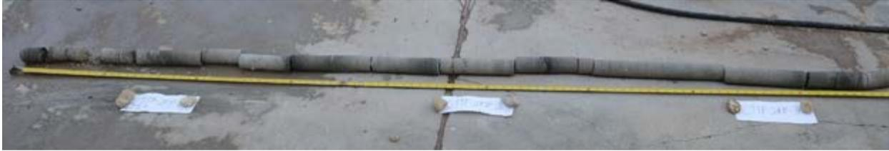
Figure 1-7: Core CTF-02FB contained 8.9 ft of limestone and shale after recovery (91% recovery).
