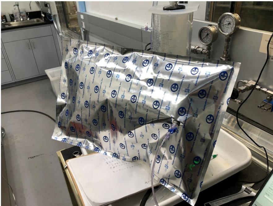
Figure 1-1: Image of inflatable bag attached to the quantitative degassing manifold used in order to capture 100% of the gas produced from the dissociation of hydrate-bearing sediment from UT-GOM2-1. Samples taken from the bag will be used to measure the bulk chemical ratios of the dissociated gases.
