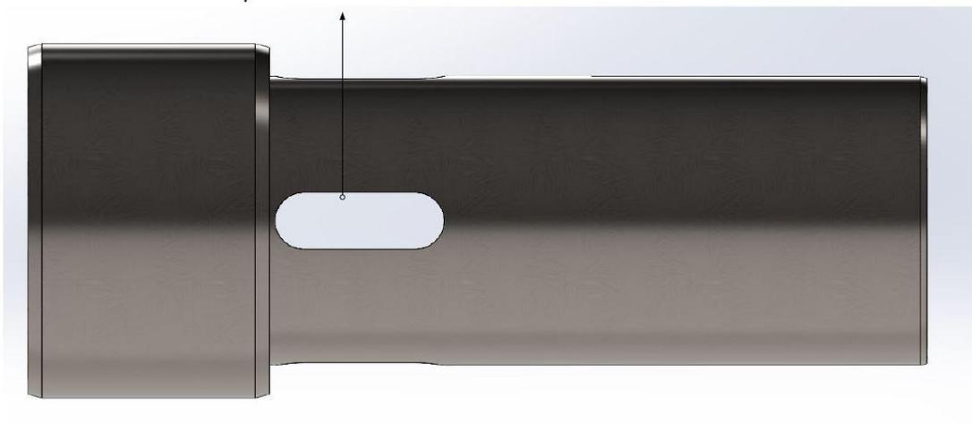
Figure 5. Modified fluid compensation ports in ball follower
