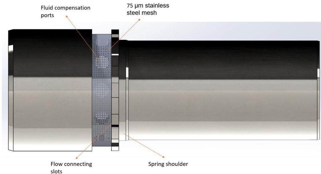
*Figure 7. Modified ball follower design including mesh filter, flow ports, spring shoulder, and connectivity slots*
