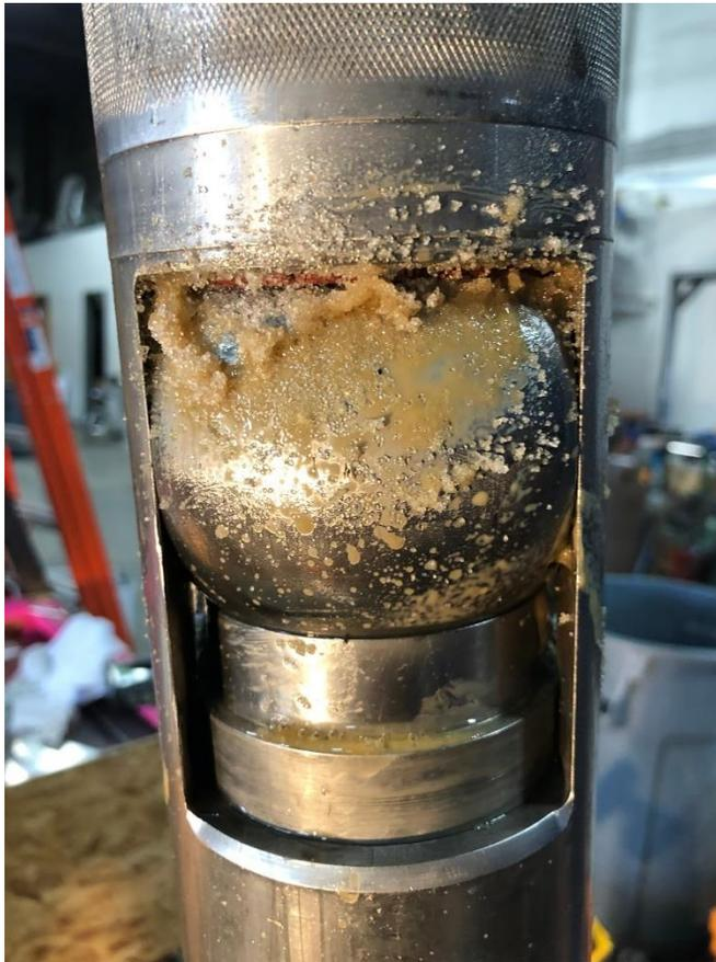
*Figure 3. Ball valve covered with #100 mesh sand*
