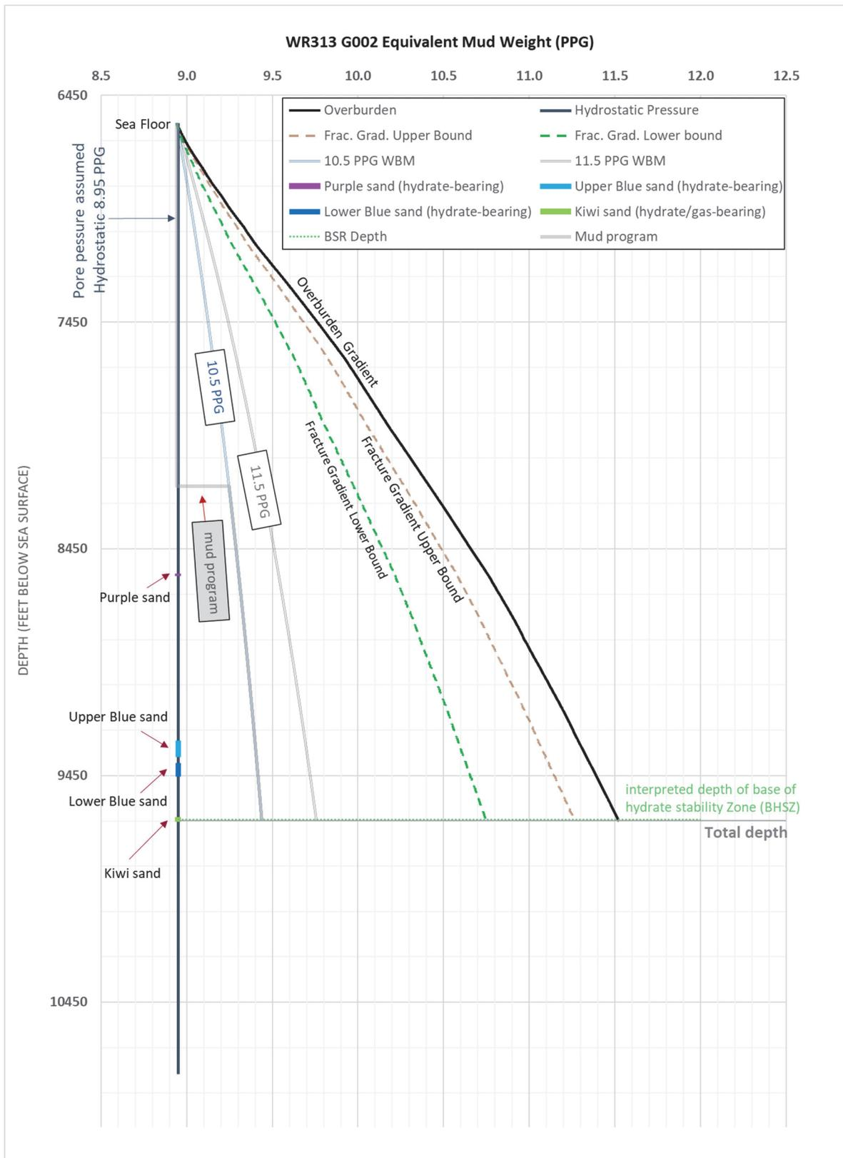
Figure 3-13. Equivalent mud weight plot for planned WR313 G002.
