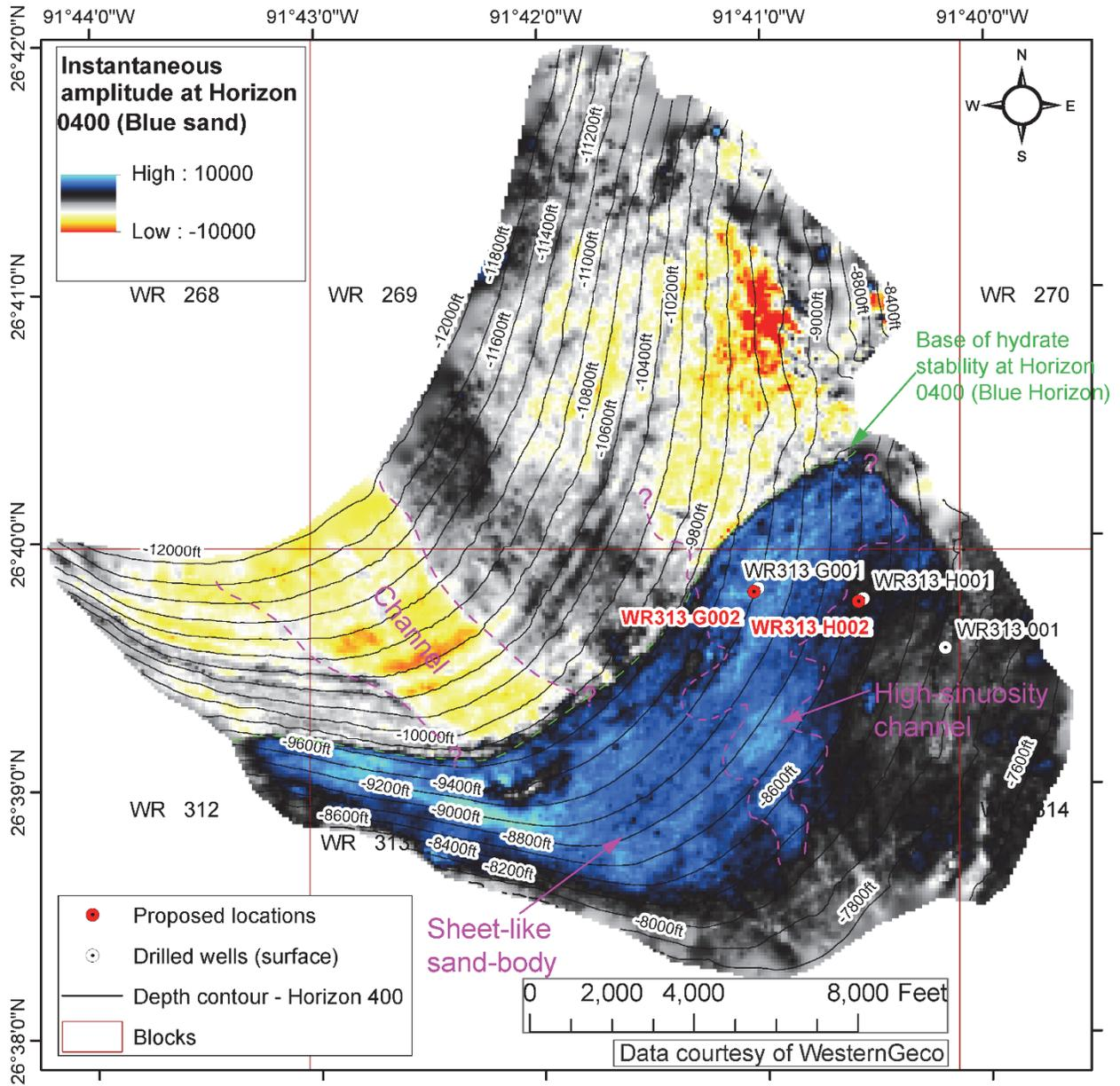
Figure 3-6. Instantaneous amplitude map extracted at Horizon 0400 (Blue Horizon) showing geological interpretation for the Blue sand – the upper of the two hydrate bearing target intervals. Maps generated from 3D seismic data used with permission of WesternGeco.
