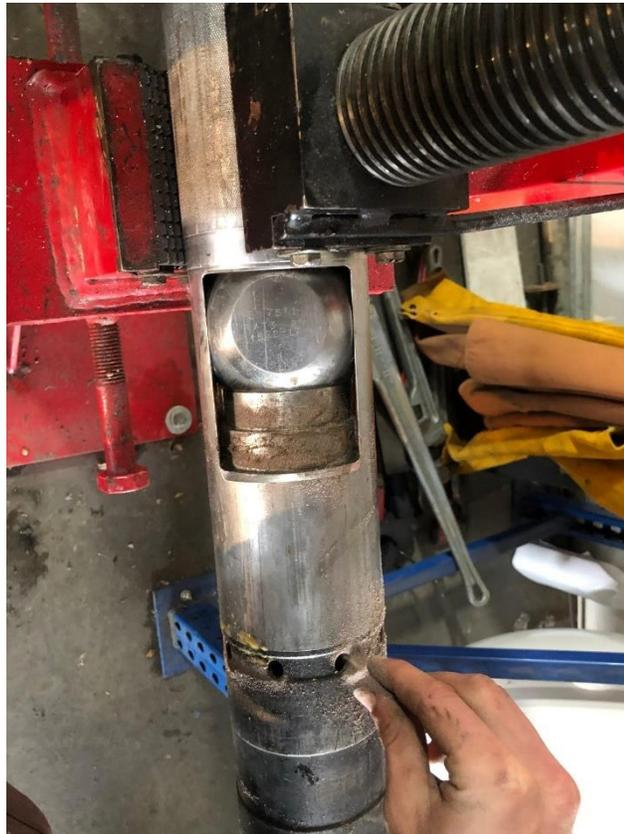
*Figure 4. Ball valve assembly with applied Aluminum Oxide*
