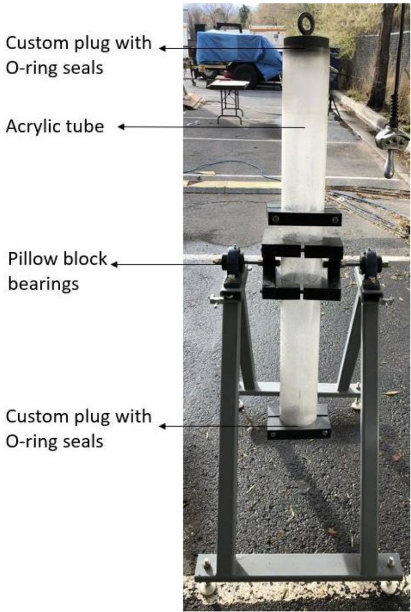
*Figure 6. Modified test fixture to allow for right-side up testing*
