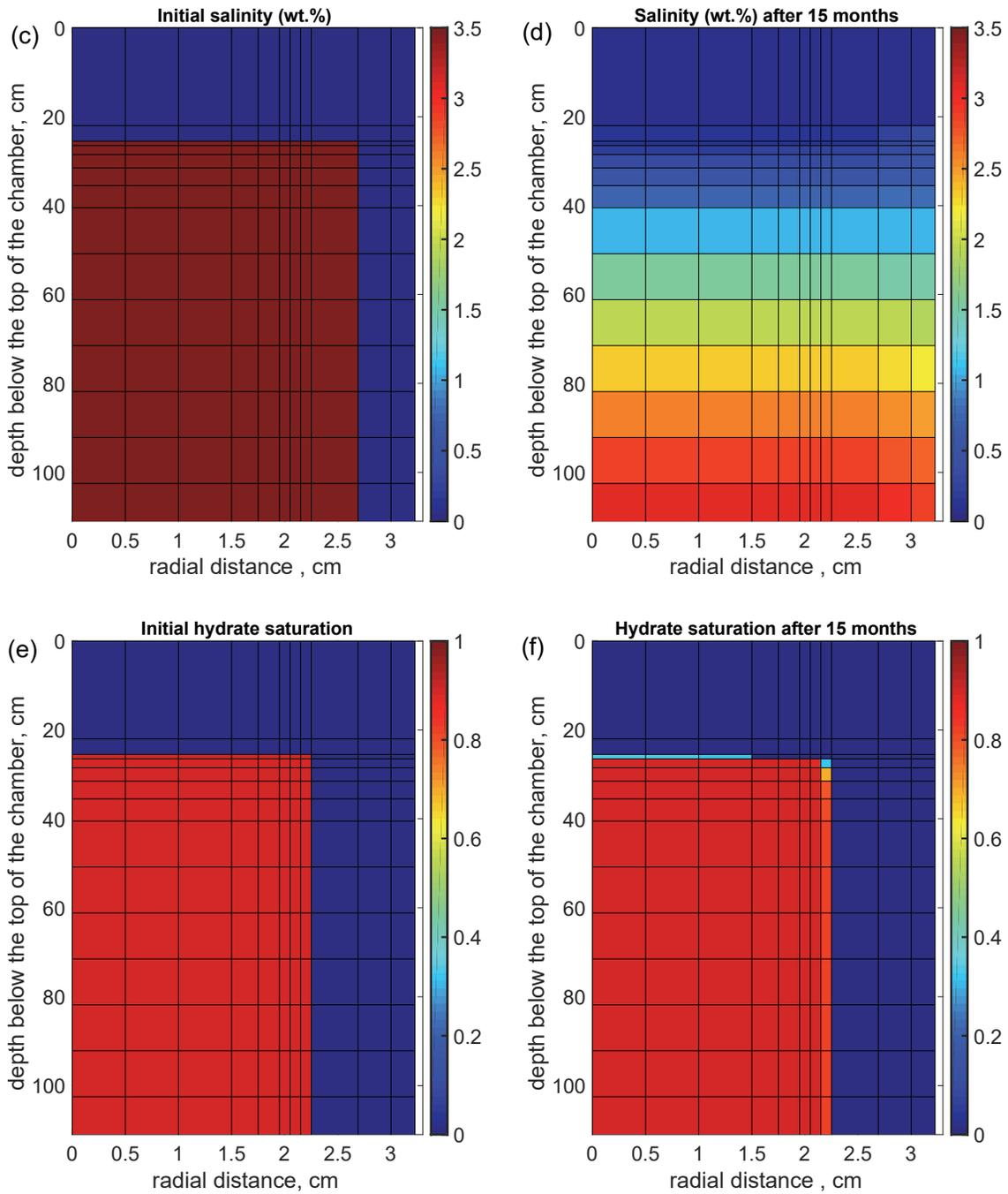
Figure 1-4. Dissolved methane concentration (a, b), salinity (c, d) and hydrate saturation (e, f) at the initial condition and after 15 months of storage at 24 MPa and 6.0 °C.
