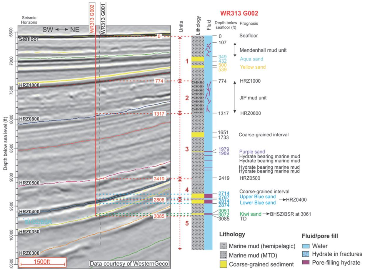
Figure 3-9. Seismic cross section DD' through Location WR313 G002 with interpreted lithology, hydrocarbon presence and major stratigraphic tops. Lithologic units (Units 1, 2, 3, 4, and 5) are marked on lithology column in red; the line of section is located in Figure 3-7.
