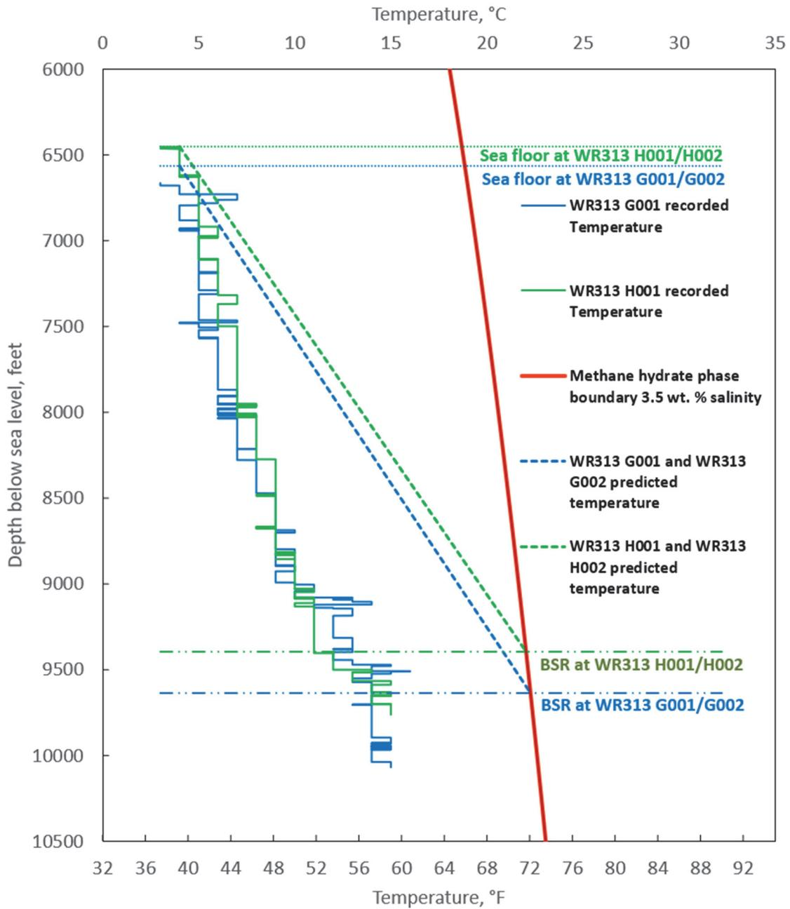
Figure 3-10. Estimated thermal gradient for WR313 G001 (blue dashed line) and WR313 H001 (green dashed line), in comparison with recorded borehole temperature (solid blue and green lines). Methane hydrate is stable on the left side of the hydrate stability phase boundary plotted in red. Horizontal lines represent interpreted base of hydrate stability zone in the wells, which intersect the corresponding predicted in situ temperature profiles at the hydrate stability phase boundary.
