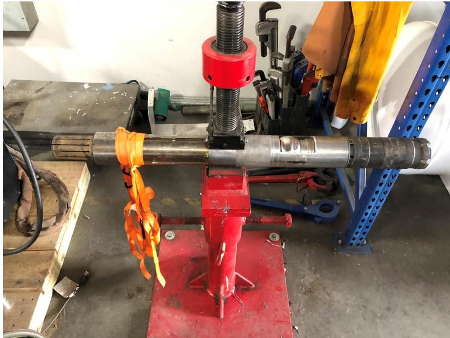
*Figure 1. Isolated ball valve assembly for dry firing*
