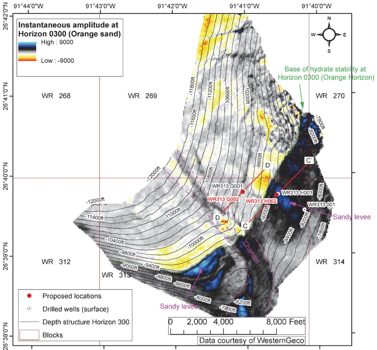
Figure 3-7. Instantaneous amplitude map extracted at Horizon 0300 (Orange Horizon) showing geological interpretation for the Orange sand – the lower of the two hydrate bearing target intervals. The well WR313 H001 and the proposed location WR313 H002 target gas hydrate-bearing sandy levee deposits showing strong positive amplitude response. Maps generated from 3D seismic data used with permission of WesternGeco.
