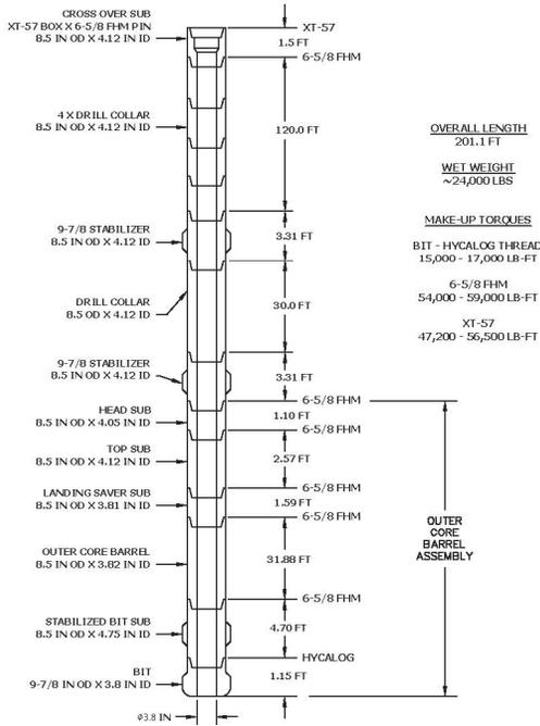
**PCTB CUTTING SHOE CONFIGURATION BHA SCHEMATIC**
