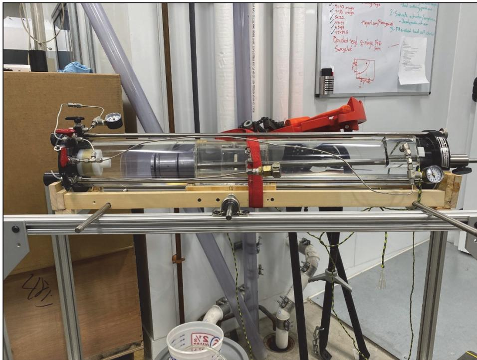
*Figure 1-5: Image of the K0 testing chamber to evaluate components that need to seal more consistently. We are able to seal the bottom cap using clean, dummy core samples. We are unable to consistently seal the bottom cap when we move to gritty pressure cores from UT-GOM2-1. Fluid communication was seen between pore fluid and actuator fluid. A variety of different seal types have been tested during pressure core tests and sealing still fails.*
