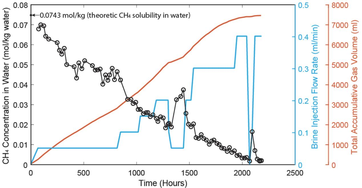
Figure 1-1: Evolution of methane dissolution during a continuous brine injection in the core sample 2FB2-1.
