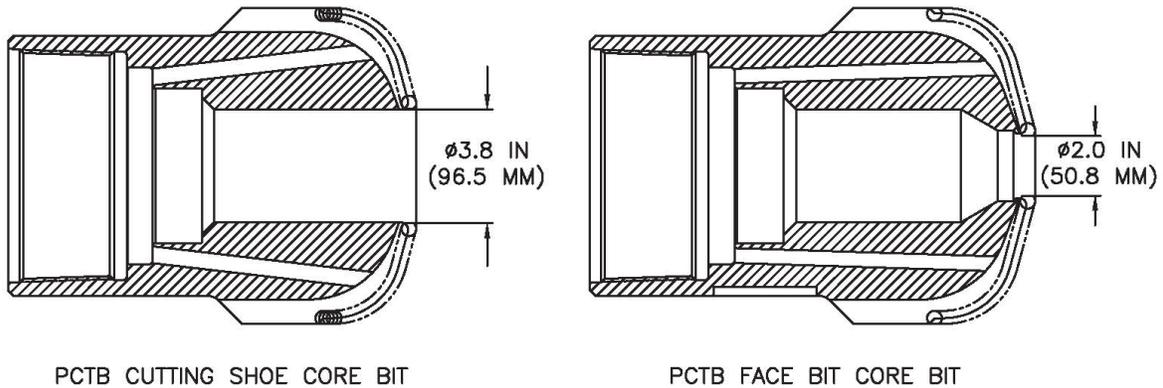
Figure 4-1. PCTB Coring Bit Configurations (Flemings et al., 2018)
