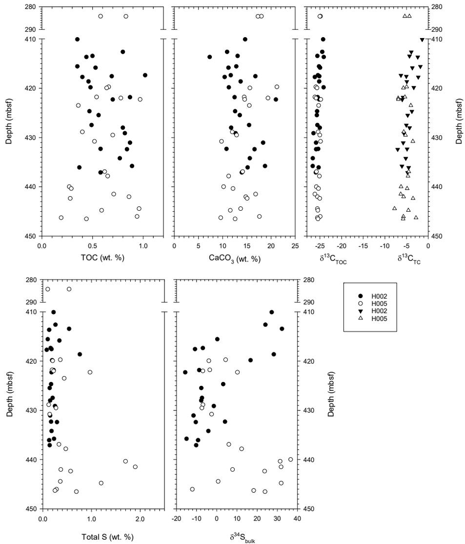
Figure 1-3: Reservoir variability in TOC, CaCO<sub>3</sub>, δ<sup>13</sup>C<sub>TOC</sub>, δ<sup>13</sup>C<sub>TC</sub>, TS, and δ<sup>34</sup>S in the GOM2 GC-955 wells H002 and H005.
