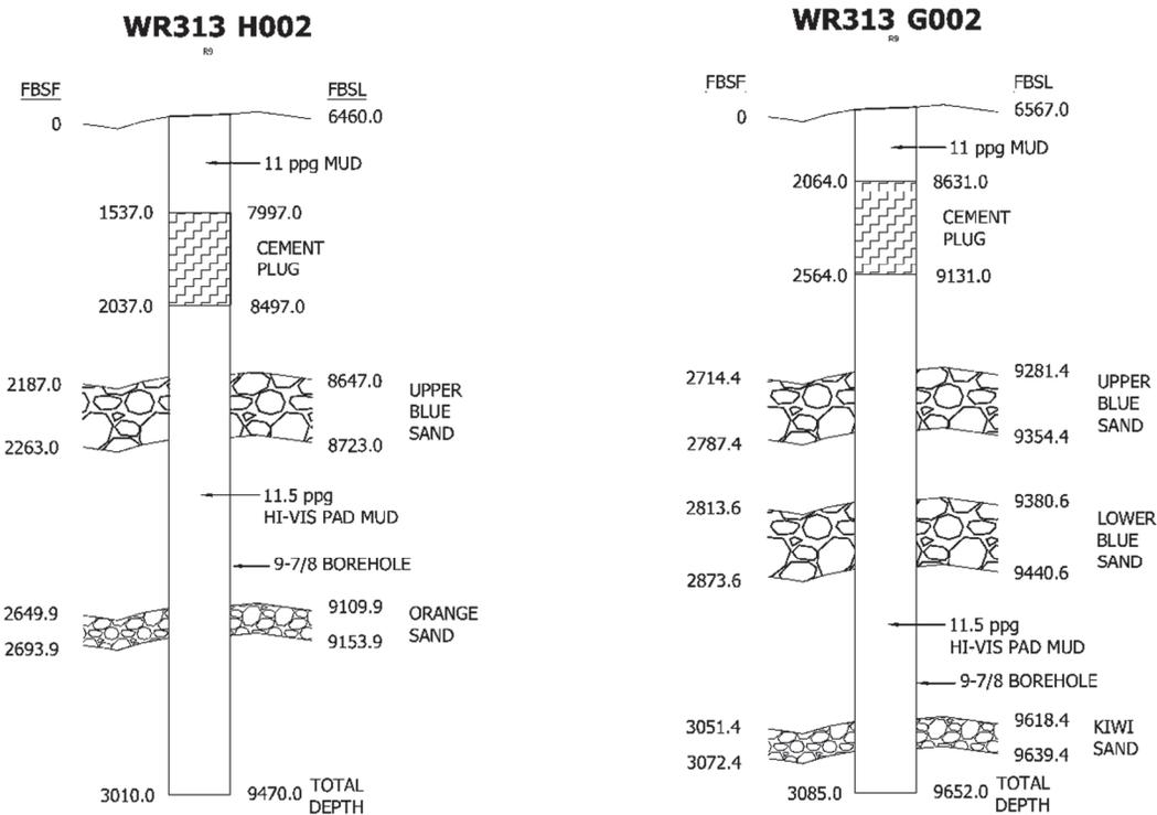
Figure 7-1. Plug and abandon cement plug emplacement hole schematics.
