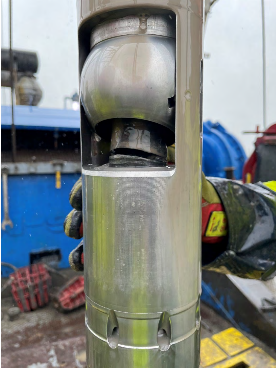
Figure 4: Coring Test 7 (COK-07CS) . Core that was not pulled up when the PCTB actuated blocked the ball from closing.
