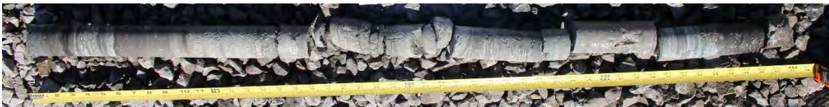
Figure 5: Coring Test 15 (COK-15FB) . 4 ft of recovered core, with the top being on the left. Interbedded shale and sand are present in the core, with the shale sections being more fragile.
