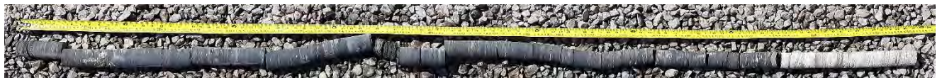
Figure 7: Coring Test 14 (COK-14FB). 8.9 ft of recovered core, with the top being on the left. The shale section was very fragile upon inspection, whereas the sand dominated section at the bottom of the core showed a more rigid behavior.
