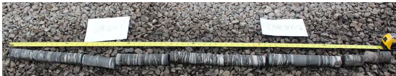
Figure 7-7. Core COK-05CS contained 5.58 ft (63.4% recovery) of interbedded shale. There are breaks in the core section, but the breaks are sharp and unrounded.
