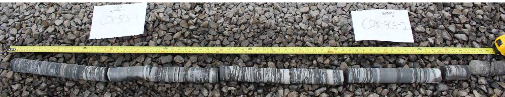
Figure 4: Coring Test 5 (COK-05CS) . 5.58 feet (67 inches) of core recovered. Good quality core with few fractures and smooth edges. Fractures appear to be from removal from core liner. Some biscuiting/fractures at bottom of core near ball valve.
