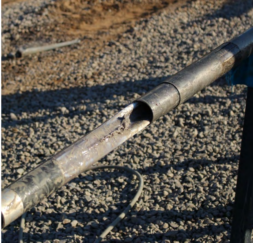
Figure 8-5. Collapsed core liner of COK-17FB. Despite the collapsed core liner, 1.1 ft of core entered the inner core barrel and was captured.
