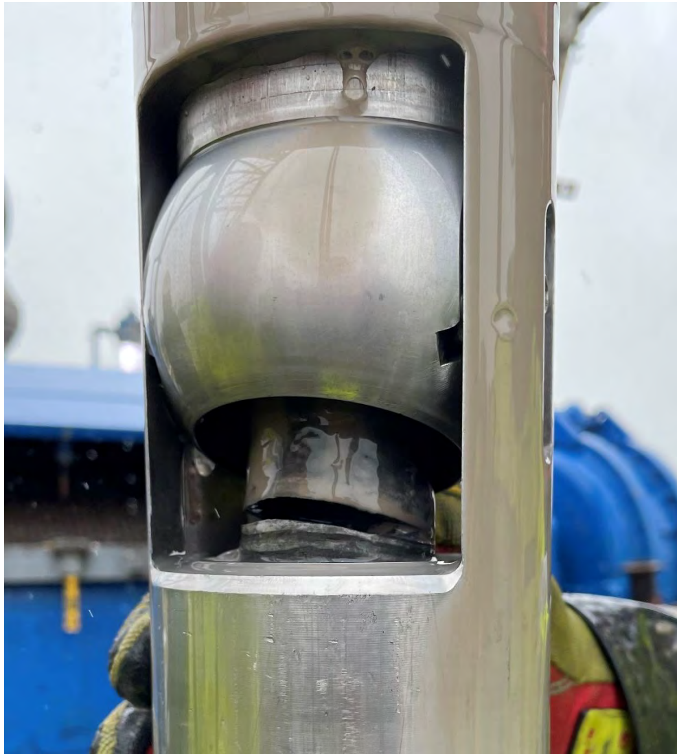
Figure 1. Jammed core on test run 7CS causing ball valve to not close
