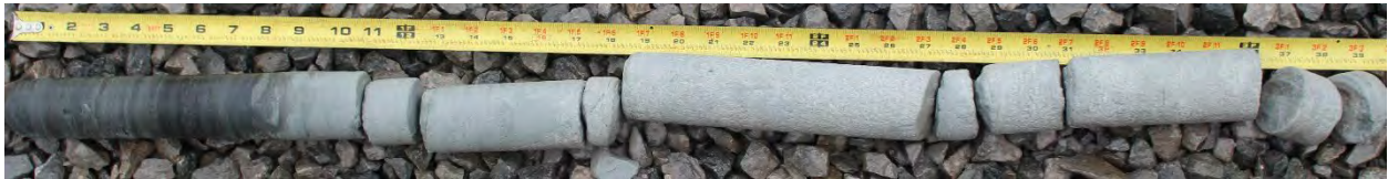
Figure 5: Coring Test 18 (COK-18FB). 3.1 ft of recovered core, with the top being on the left. Interbedded shale and sand are present in the core, with the shale sections being more fragile.
