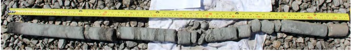
Figure 6: Coring Test 16 (COK-16FB) . 4.4 ft of recovered core, with the top being on the left. Shale is the predominant lithology throughout the entire core.
