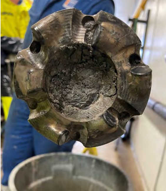
Figure 8-2. The jammed cutting shoe of test COK-07CS, seen from the bottom.
