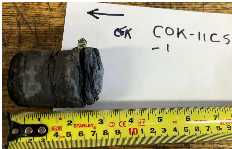
Figure 7: Coring Test 11 (COK-11CS). 3” of recovered core. The core was very fragile upon inspection.
