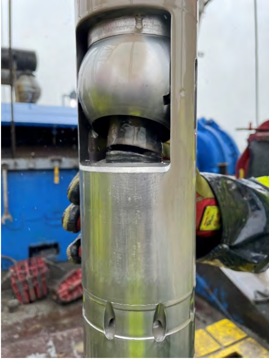
Figure 8-1. In test COK-07CS, a small length of core was jammed in the cutting shoe and protruded up through the ball valve, preventing it from closing.
