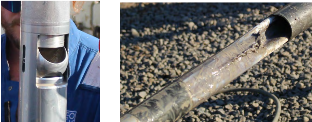
Figure 9: Coring Test 17 (COK-17FB) . Partial ball valve closure observed at the drilling floor (left) and collapsed core liner.
