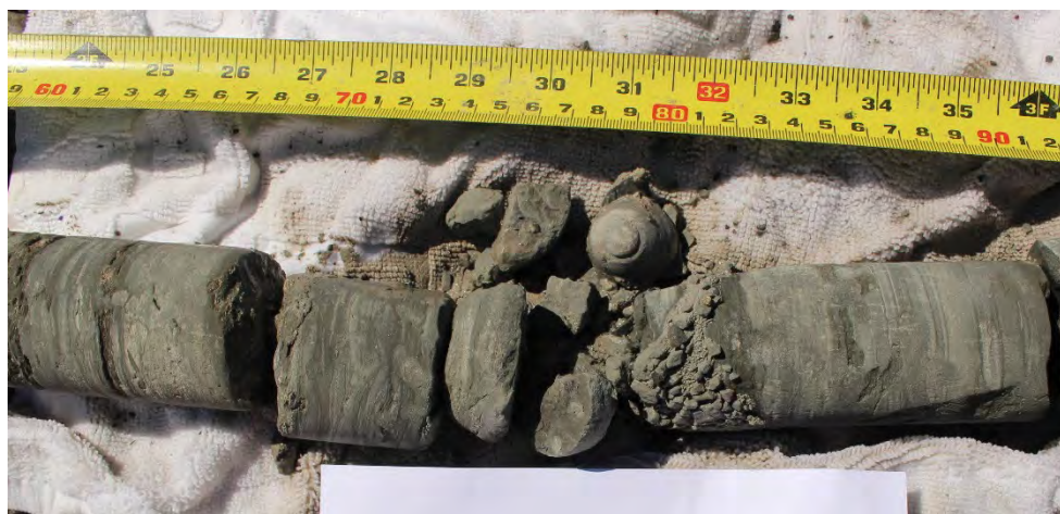
Figure 7-8. Clear evidence of biscuiting in core COK-15FB. The lithology of this core is sandier than most of the other cores.
