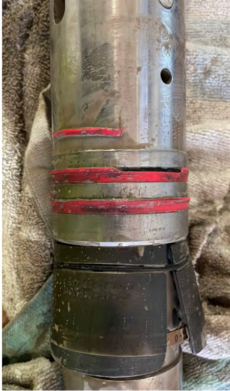
Figure 8-3. COK-09CS failed to seal and actuate properly due to a damaged plug seal on the upper end of the inner core barrel. The damaged seal is shown here after post-deployment disassembly.
