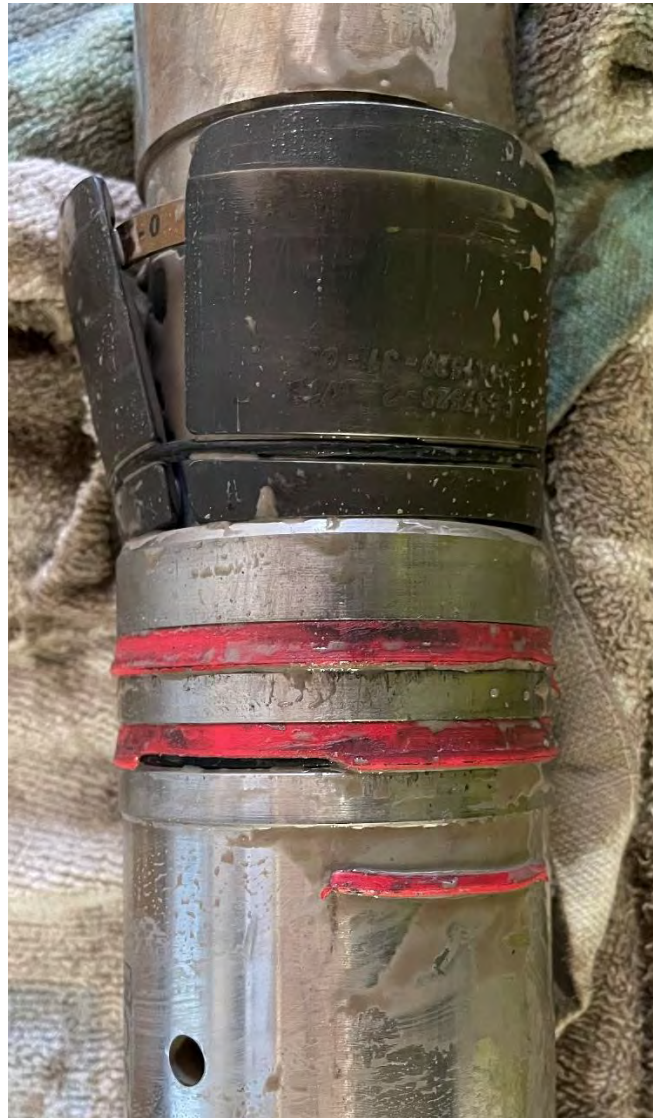
Figure 3. Damaged IT plug polypak seal causing jamming of the tool during actuation
