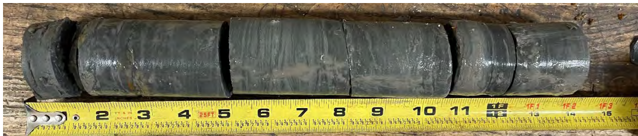
Figure 10: Coring Test 17 (COK-17FB) . 1.16 ft of recovered core from the core liner, despite partial collapse.
