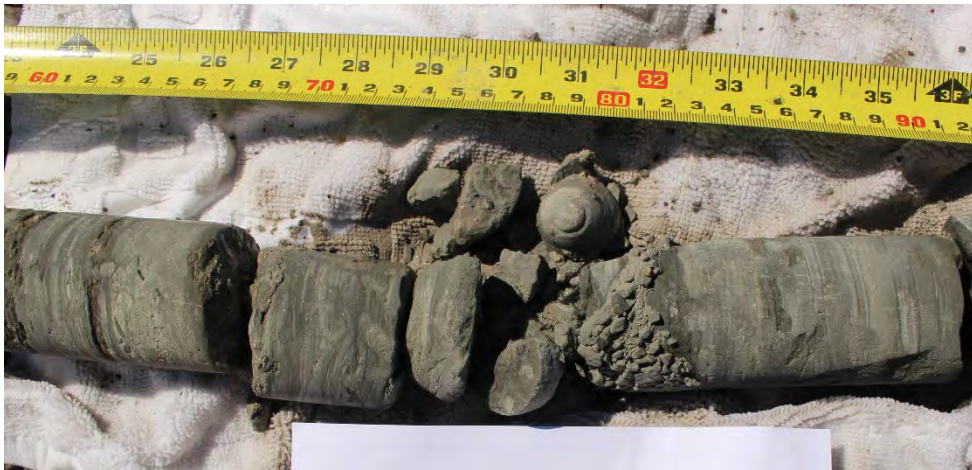
Figure 7-8. Clear evidence of biscuiting in core COK-15FB. The lithology of this core is sandier than most of the other cores.
