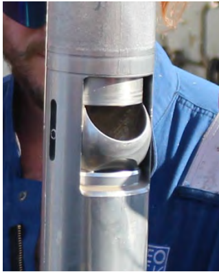
Figure 9: Coring Test 17 (COK-17FB). Partial ball valve closure observed at the drilling floor (left) and collapsed core liner.
