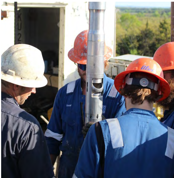
Figure 8-4. Upon retrieval of COK-17FB, the ball valve was visibly open.
