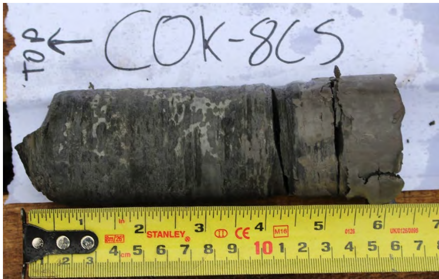
Figure 4: Coring Test 8 (COK-08CS) . 6" of jammed core.
