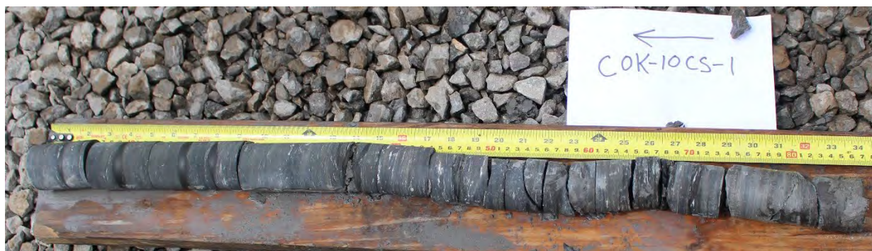
Figure 5: Coring Test 10 (COK-10CS). The 34" of recovered core was very fragile upon inspection. Shale is the predominant lithology.
