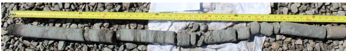
Figure 6: Coring Test 16 (COK-16FB) . 4.4 ft of recovered core, with the top being on the left. Shale is the predominant lithology throughout the entire core.
