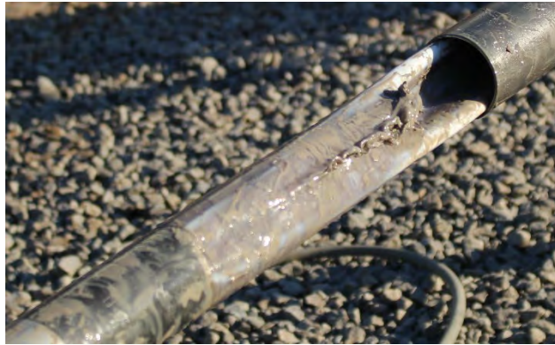
Figure 9: Coring Test 17 (COK-17FB). Partial ball valve closure observed at the drilling floor (left) and collapsed core liner.
