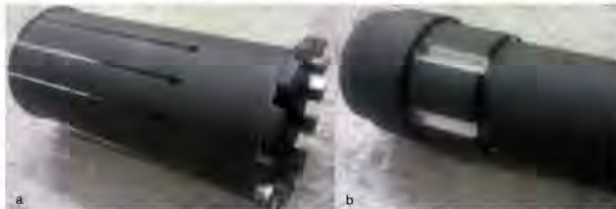
Figure 1. Flow slots added to the Ball Valve Release Collet (a) and to the Ball Follower (b).
