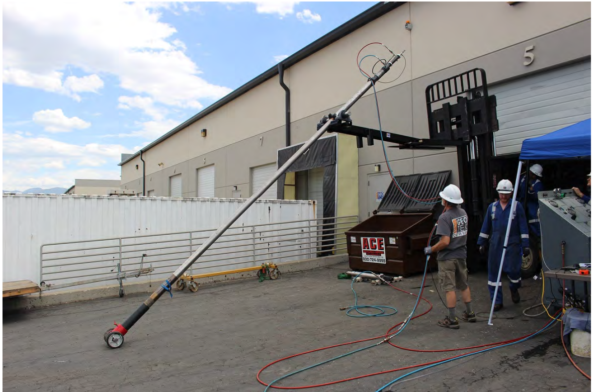
Figure 2, VFFPT Test Fixture being raised to vertical position for test.
