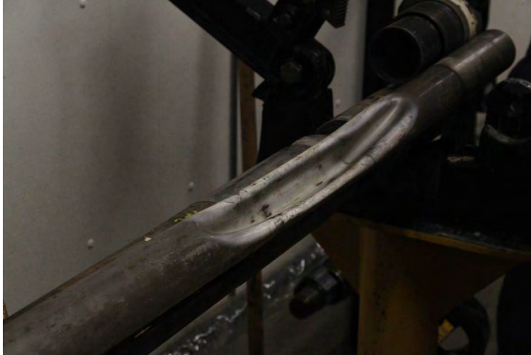
Figure 4: Collapsed liner after Flow Test 3.
