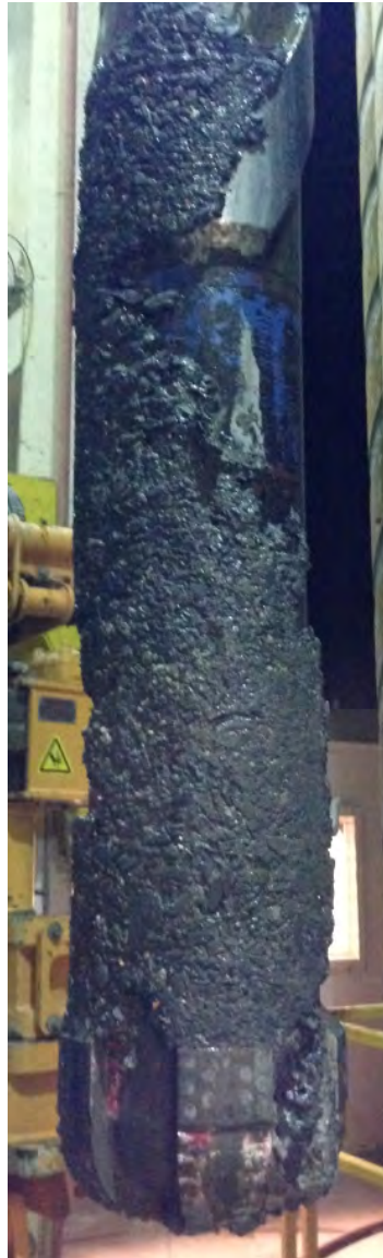
Figure 7. BHA with cuttings balling up after POOH after Core #8.
