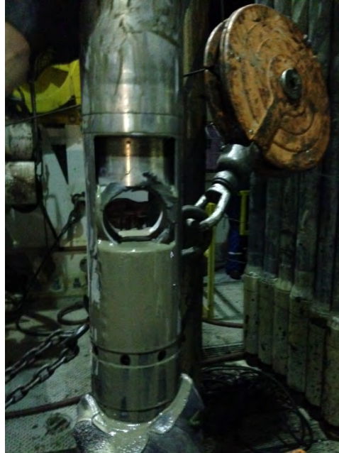
Figure 5. PCTB ball valve coming out of hole after Core #2 – closed but not holding pressure.
