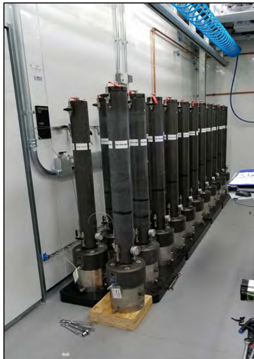
Figure 3-1: Pressure cores at refrigerated UT Pressure Core Center
