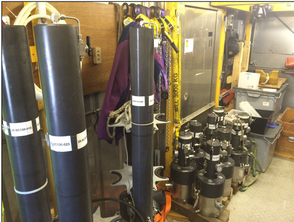
Figure 0-3. Image of 1.2 m and 0.35 m storage chambers on-board in Geotek cold storage
