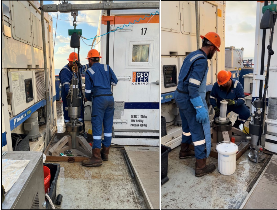
Figure 1: PCTB-CS pressure core sample from Hole UT-GOM2-2-H003 being converted to a liquid nitrogen frozen microbiological cryo core, which will be stored in an -80°C freezer on the Q4000.
