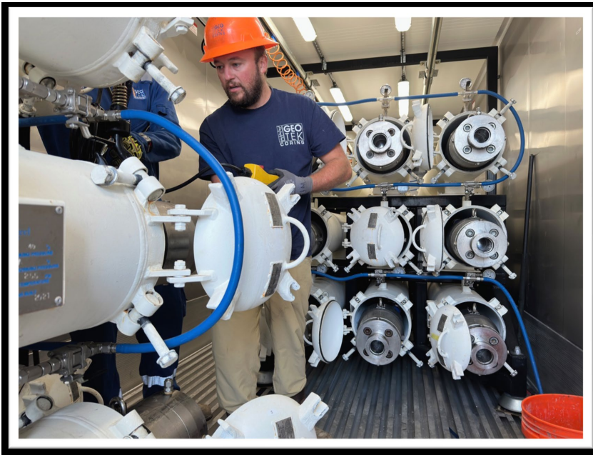
Joey (Geotek) loading the 17 pressure from the GOM2-2 expedition into the PTRANS36. This 40' specialized Geotek unit, with 36 overpacks, is a DoT certified system for transporting pressure cores which contain flammable gas in hydrate form. Cores were transferred to UT on Sept 9 and then remaining pressure cores were delivered to Salt Lake City.
