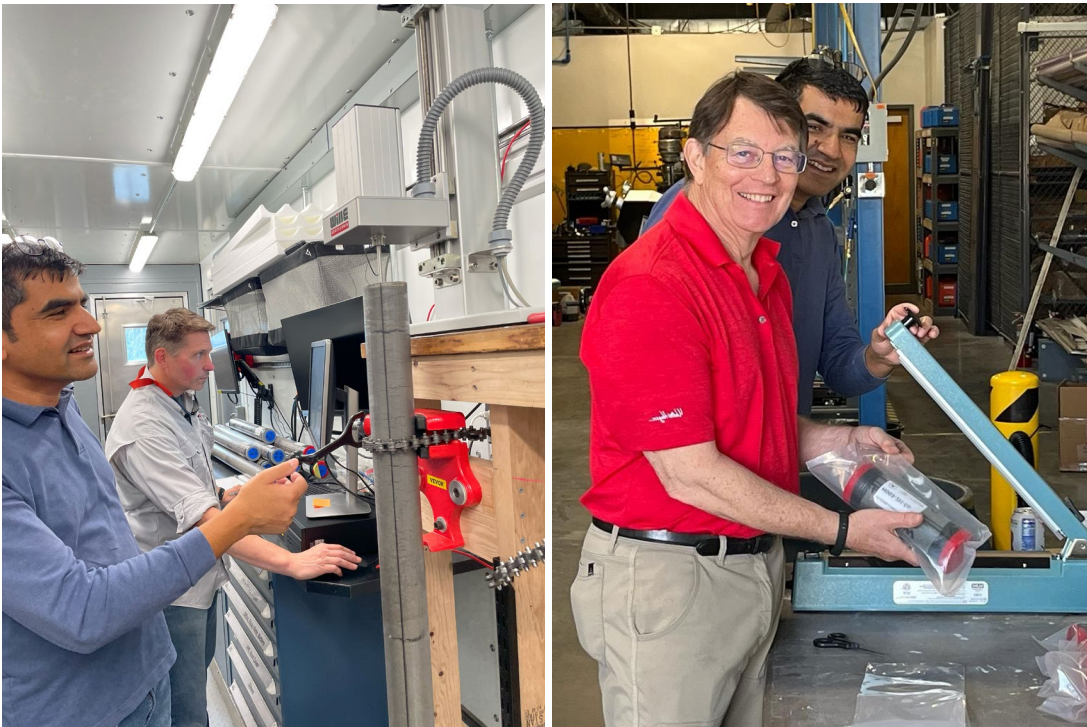
Figure 1: Left: Athma Bhandari (U.T.) clamps a sample being measured for undrained strength with a Table Vane. The measurements tell us about the sediment's material properties. Derek Sawyer (Ohio State) drives the software for the analysis. Right: Jack Germaine (Tufts University) proudly demonstrates a whole core sample preserved for later geomechanical analysis.
