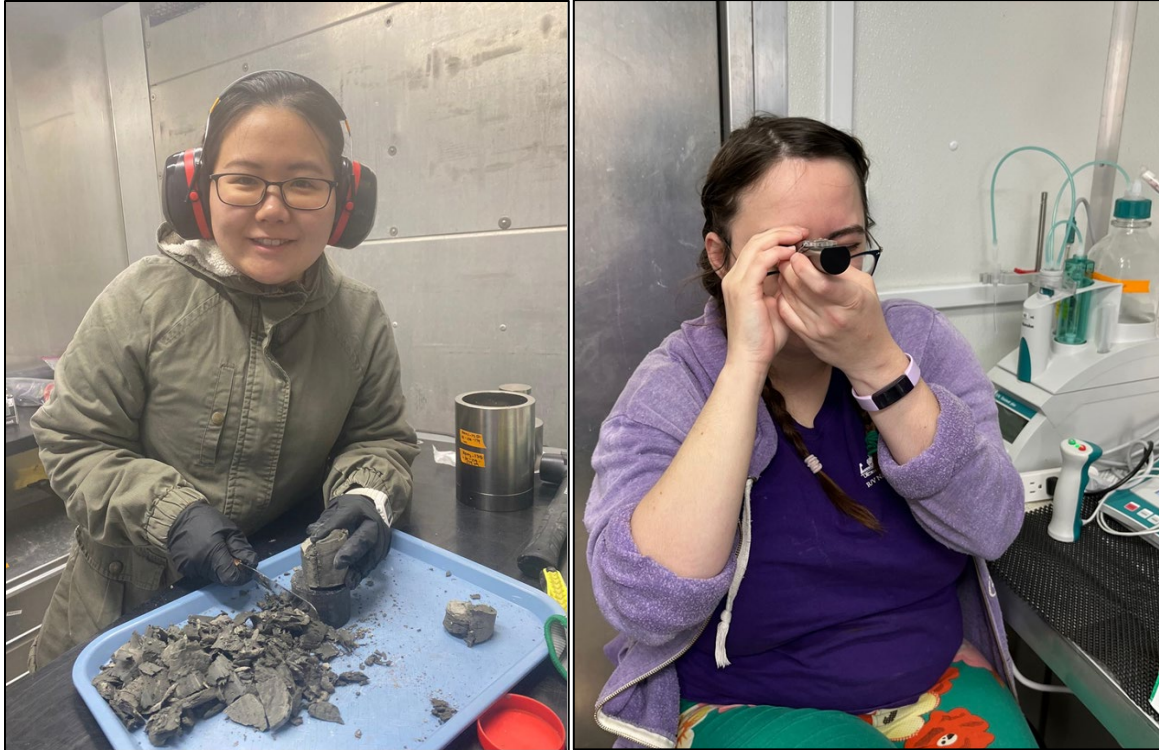
University of Washington researchers working in the pore water labs. Left: Man-Yin Tsang prepping a sample for pore water squeezing in the Pore Water Reefer. Right: Taylor Walton making a refractometer measurement.
