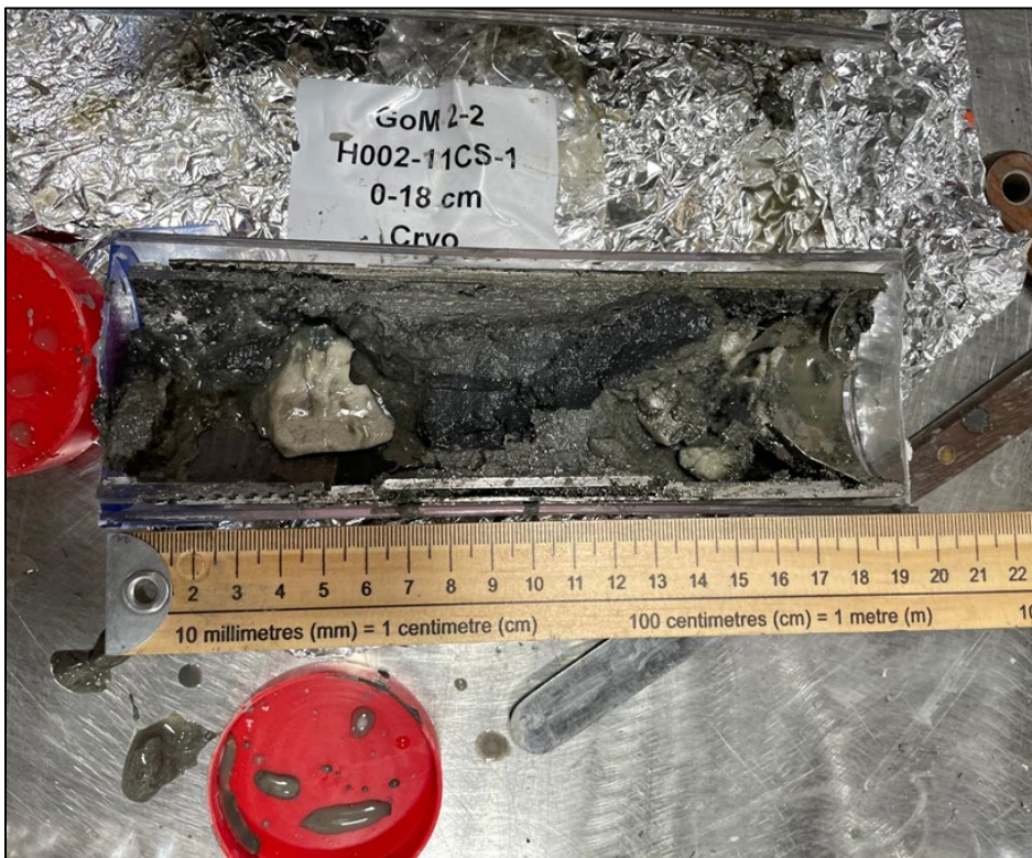
Gas Hydrate (white chunks) in core section H002-11CS-1 from pressure core H002-11CS cored from the Orange sand. This section was cryogenically frozen before depressurization. The section was then kept at -80 C until it was sub-cored for cell counts and DNA extraction at Salt Lake City.
