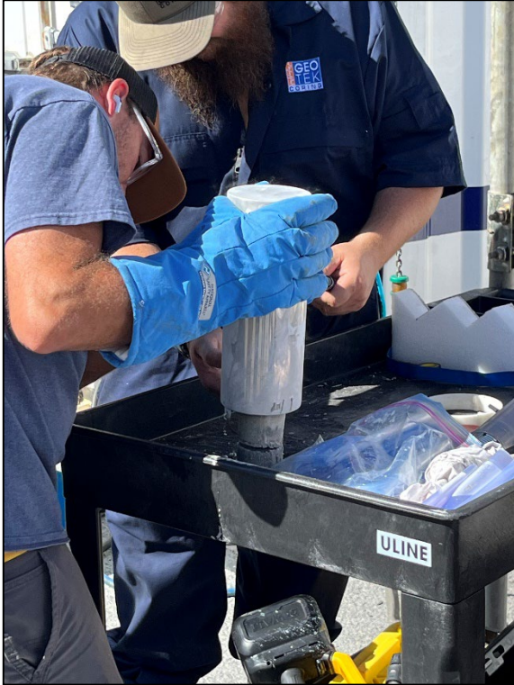
Geotek Extracting a cryo-core from the liquid nitrogen depressurization chamber
