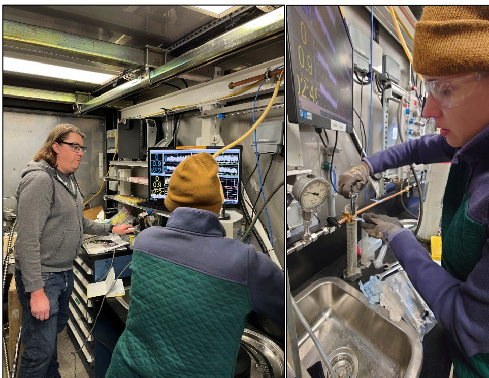
Steve Phillips (USGS) and Rachel Coyte (Ohio State) measuring the volume of produced gas and capturing gas samples for assessments of dissolved gases, hydrate saturation, and gas composition including hydrocarbons, isotopes of Carbon, and Nobel gases.
