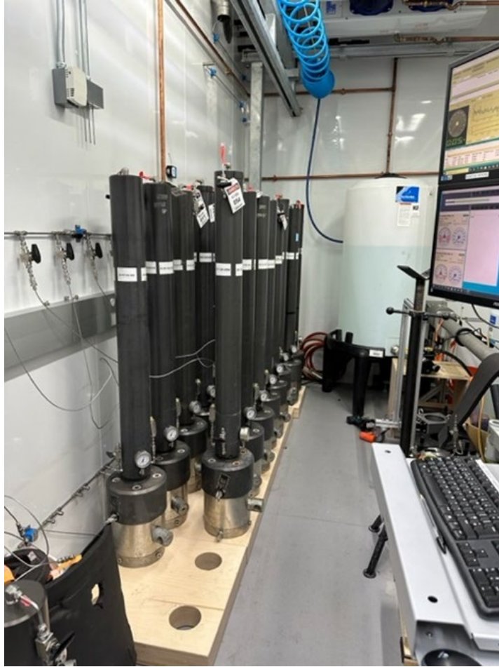
Figure 1-2. Thirteen pressure cores from UT-GOM2-2 (WR313) and four from UT-GOM2-1 (GC955) stored in Geotek SC120 containers on quad bases in the UT Pressure Core Center.
