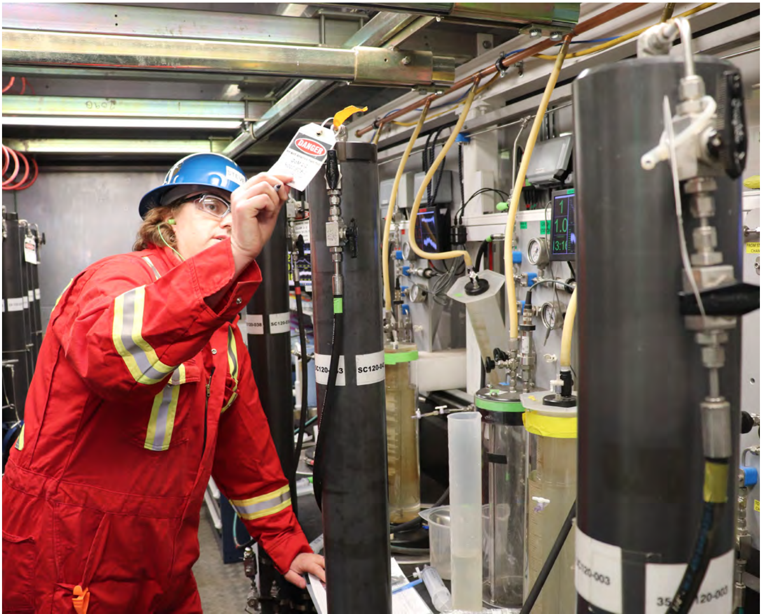
USGS scientist Stephen C. Phillips degassing pressure cores — a process that measures how much gas is in each core sample. Photo Credit: Monica Kortsha
