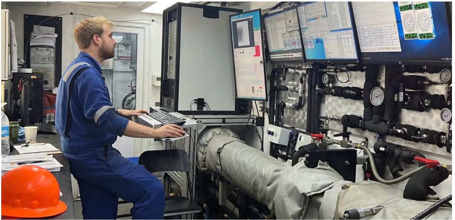
Geotek Ltd. scientist Andrew Goodridge watches several output monitors while the Geotek pressure core and transfer system (PCATS) logs and images a pressure core. Photo credit: Geotek Ltd.
