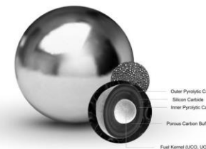
Figure 5: Visual model of the TRISO fuel pellet
