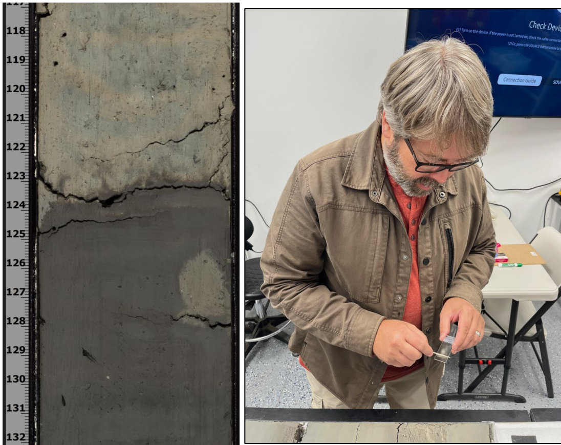
Figure 1-4. Core Section H003-14H-1 top at 80.8 mbsf with possible sequence boundary. Lighter colored area at 127 cm within the darker lithogenic clay (123.5 cm and lower) is indicative of a burrow dug by an organism and later filled with lighter-color overlaying biogenic-pelagic ooze (123.5 cm and higher). Right, photo of UNH PI Joel Johnson preparing a smear slide in Salt Lake City.
