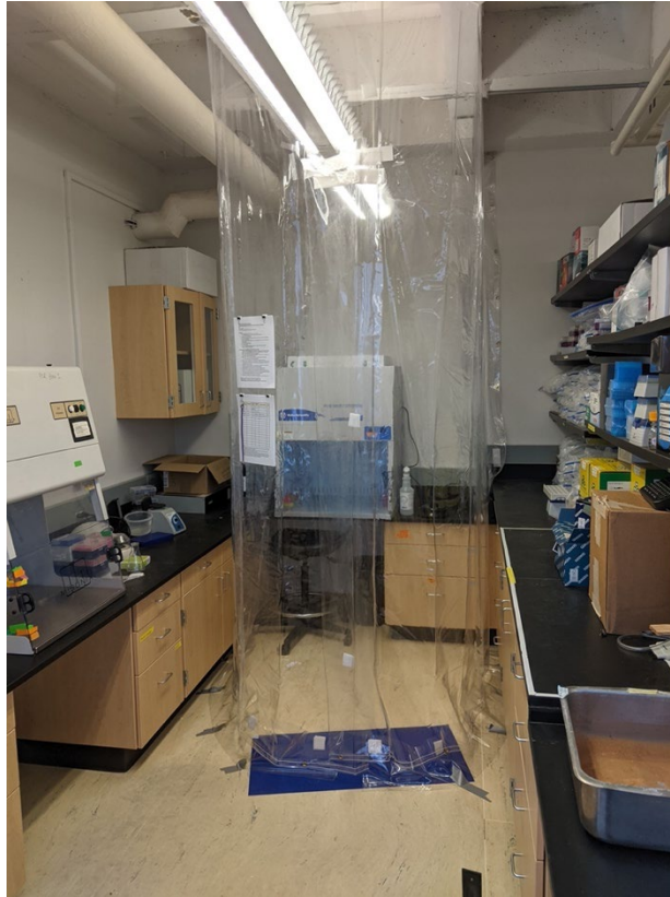
Figure 1-11. Enclosure in OSU Geomicrobiology lab designed to minimize lab-borne contaminants during processing of GoM2-2 samples
