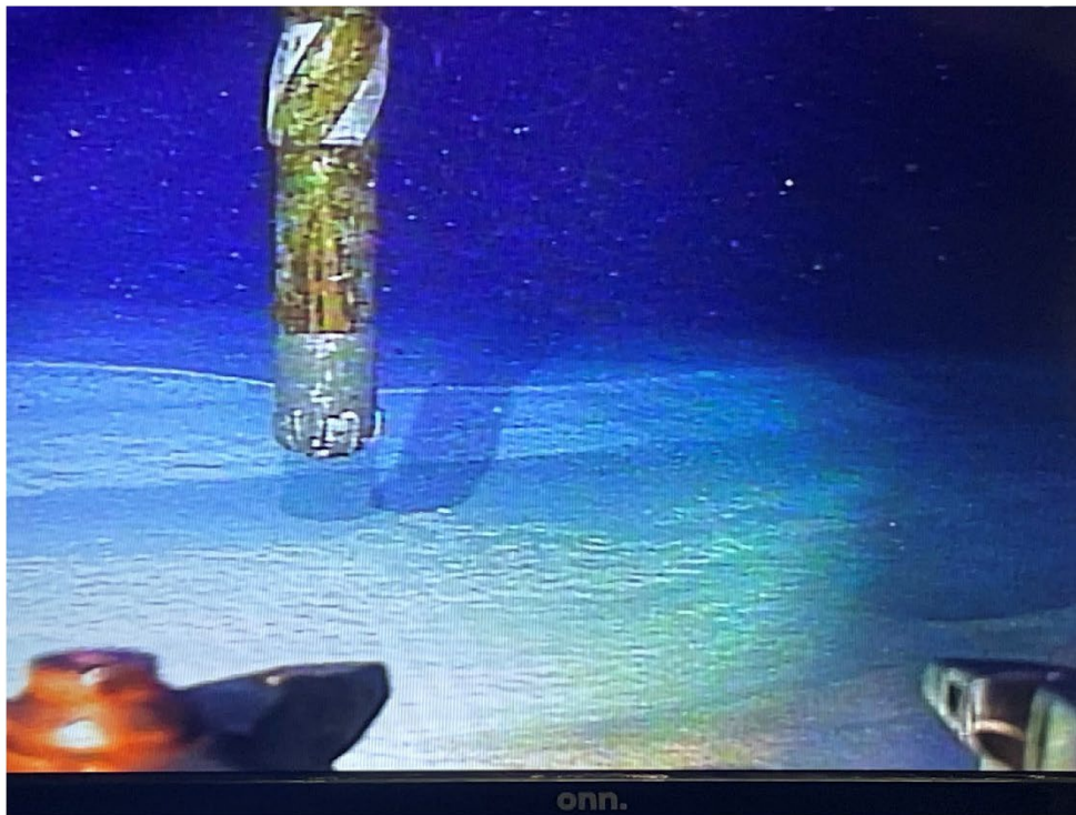
Figure 1: Helix D/V Q400 ROV acquired image of the re-entry into Hole UT-GOM2-2-H002 . Visible is the edge of the crater like feature that marked the location of the expected well head at the seafloor; note the lack of any well head like features that was ultimately proven to be the surface location of the hole.
