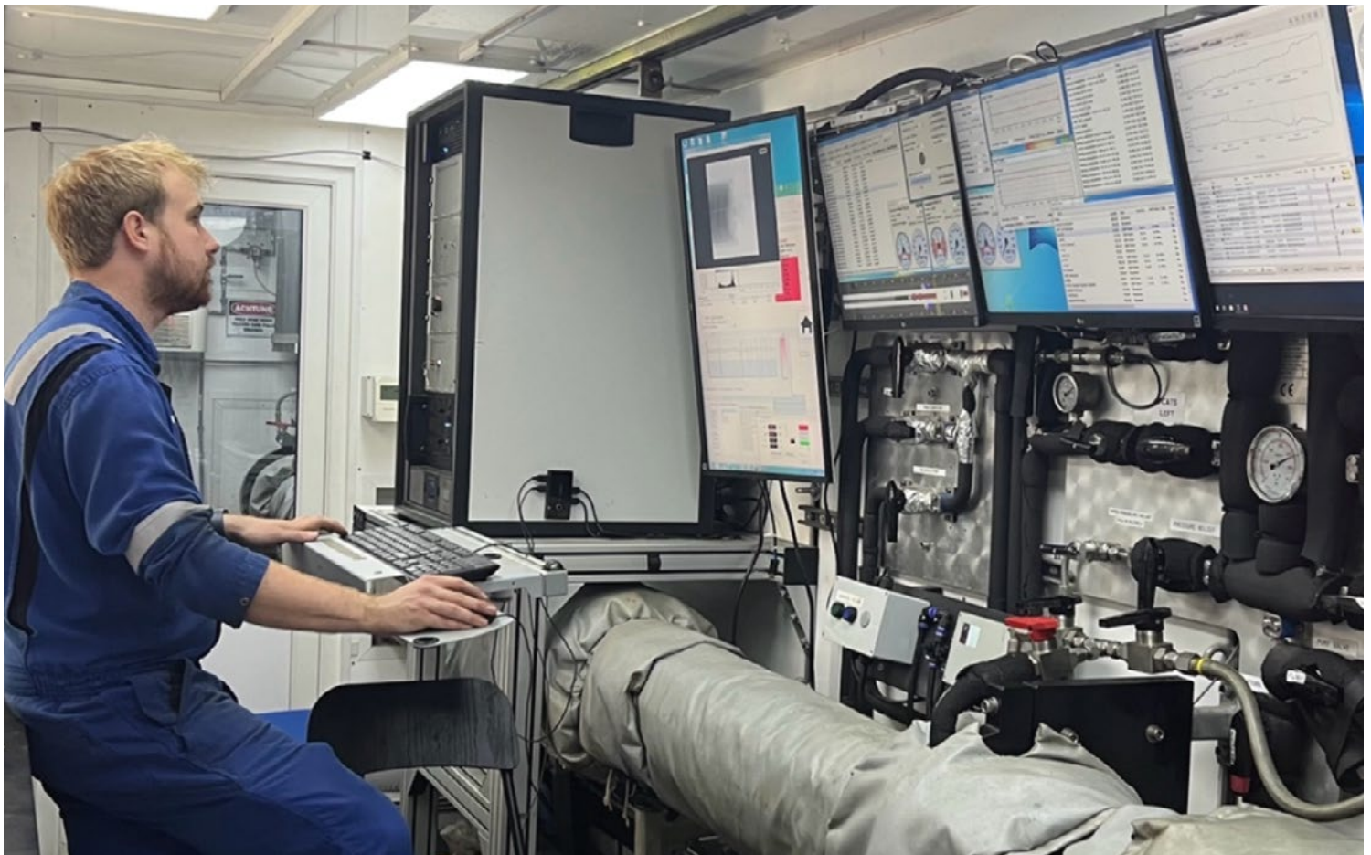
Geotek Ltd. scientist Andrew Goodridge watches several output monitors while the Geotek pressure core and transfer system (PCATS) logs and images a pressure core. Photo credit: Geotek Ltd.
