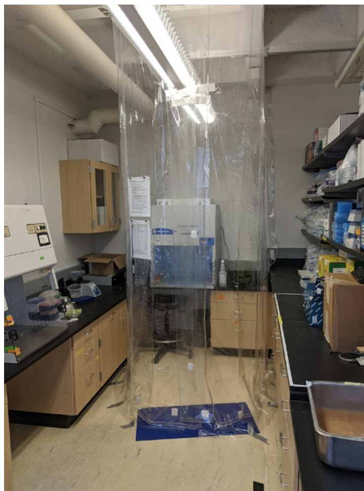
Figure F56: “Greenhouse” enclosure in Geomicrobiology lab at Oregon State University designed to minimize lab-borne contaminants during processing of GOM2-2 samples.
