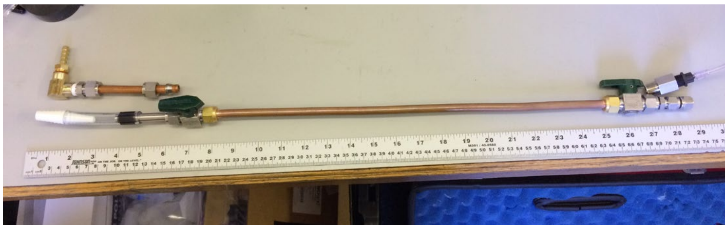
Figure F62: Copper tube with Swagelok valves for noble gas sampling.
