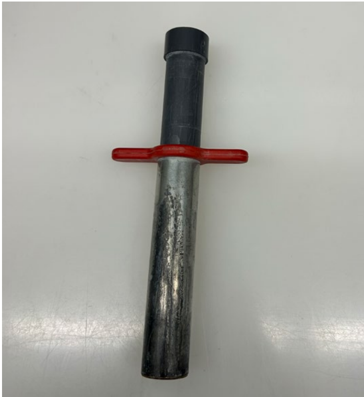
Figure F44: Photos of the brass plug corer and plunger used to extract moisture and density (MAD) samples from the split core working half.
