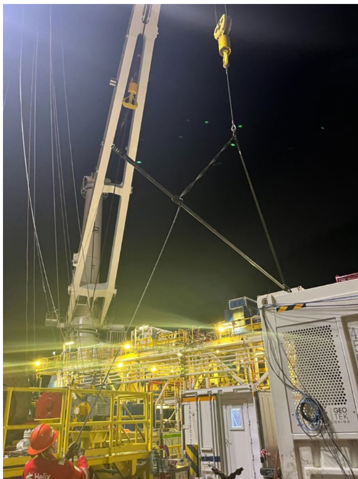
Figure F15: Image of the lower part of the Advanced Piston Corer conventional coring tool being moved from the drill floor to the Geotek Core Receiving mobile lab.
