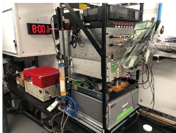
Figure F66: USGS Auto-SIM GC/CRDS System with attached Cali-5 gas bags. The Auto-SIM distributes gas to the USGS DSIM and GC. Gas composition is measured by the SRI MG#5 GC. Methane/CO 2 stable carbon isotopes are measured by the Picarro G2201-i CRDS.
