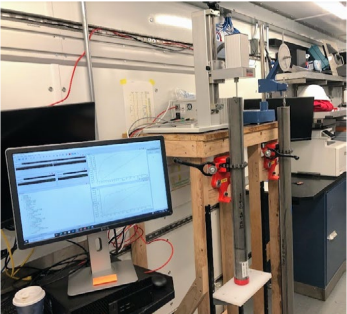
Figure F52: Two core sections mounted on the adjustable frame being tested with the fall cone penetrometer (right side) and automated vane shear device (left side) with connected computer and display.
