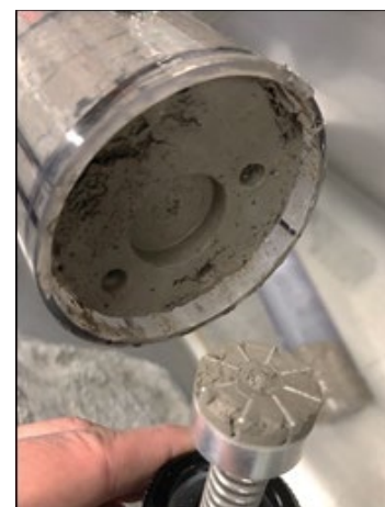
Figure F49: (left) Diagram of testing locations for handheld vane shear and pocket penetrometer made onboard on conventional piston cores (diameter = 2.4 inches (60.9 mm)) and pressure cores (diameter = 2 inches (50.8 mm)). Vane shear was measured first in the center of the core (measurement code VANE). Pocket penetrometer measurements were made in the available space around the vane location and away from core edges (measurement code PEN). Photo shows the vane shear device and an Advanced Piston Core (G-APC) section after VANE and PEN measurements.
