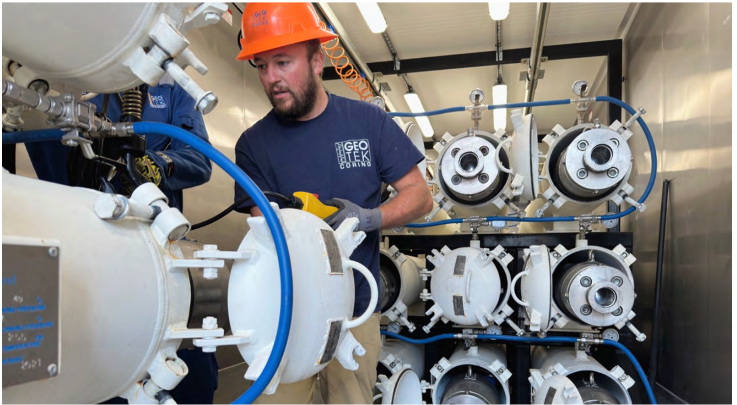
Dan Minarich prepares the Geotek overpack system used to transport pressure cores over land to UT. Photo credit: Geotek Ltd.
