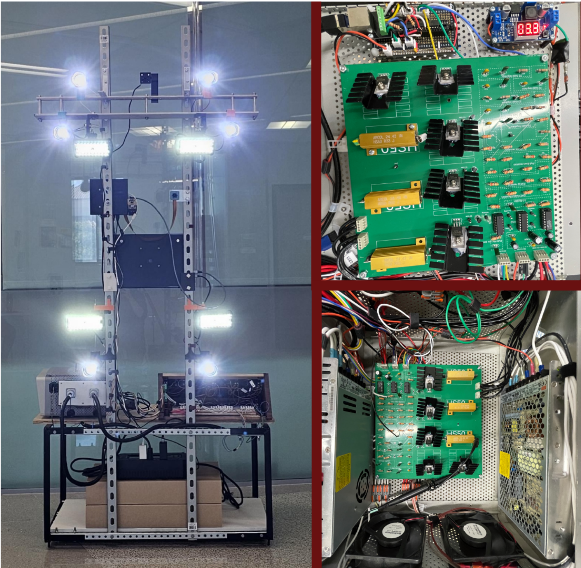
Left: Lighting arrays with UPS, enclosure, cameras, and switching controls. Right: Inside view of drive electronics, power supplies, and thermal management nested in the ICLS drive electronics enclosure.
